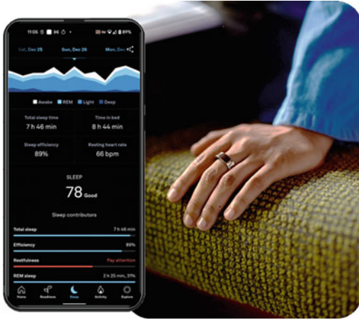
Fig. 21.16 Subject wearing a commercially available ring sensor (right, picture from Oura Health Oy) that provides measures of sleep quality via the companion smartphone application (left). Sleep quality is relevant to stroke rehabilitation in many ways, including the impact on the consolidation of motor gains
