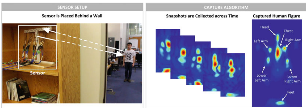
Fig. 21.14 Radar-like systems can provide a totally unobtrusive way to monitor patients’ position in the home environment and hence infer contextual information of great use in home-based interventions. The sensor (left panel) consists of a radio transmitter/receiver array. The
