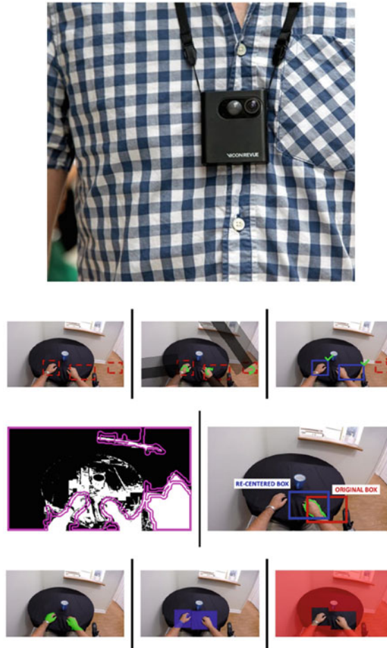
Fig. 21.13 A wearable camera (left panel) can be utilized as an alternative to wearable sensors to detect UL motor activities (right panel). Reproduced with permission (Vicon Revue camera picture courtesy of Oxford Metrics, UK—left panel; Likitlersuang et al. ( https://doi.org/10.1186/s12984-019-0557-1 , licensed under CC BY 4.0)—right panel)
