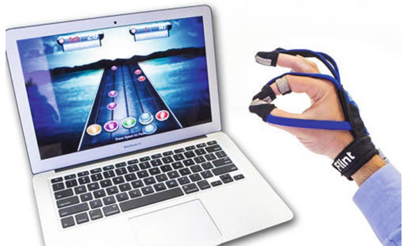
Fig. 21.4 The MusicGlove is a system that integrates wearable technology and an interactive game (e.g., the Guitar Hero ) to train hand dexterity. Reproduced with permission from Flint Rehabilitation Devices, LLC
