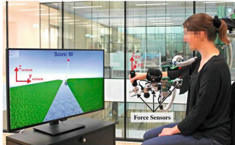
Fig. 27.13 Improved haptic rendering performance thanks to additional force sensors measuring the interaction force between the user's arm and the robotic device. The picture shows an inverted pendulum task using the ARMin exoskeleton as a visuo-haptic interface (Copyright IEEE, with permission).
