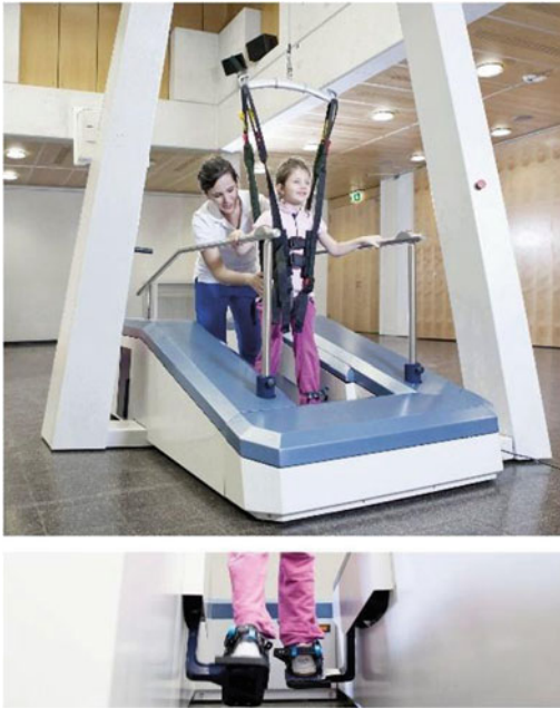
Fig. 14.6 LYRA. The end-effector THERA-trainer LYRA (THERA-Trainer by medica Medizintechnik GmbH, Hochdorf, Germany) allows to train children and youths with body heights varying between 1.00–1.95 m and a body weight up to 150 kg. The patient is positioned on footplates, and step lengths can easily be adjusted from 39 to 67 cm according to the patient's need. Foot bindings are interchangeable, taking into account different shoe sizes and different step widths. Pediatric handrails can be mounted onto the handrails supporting the younger patients, and additional hip stabilization is available in various sizes. Picture with kind permission from THERA Trainer
