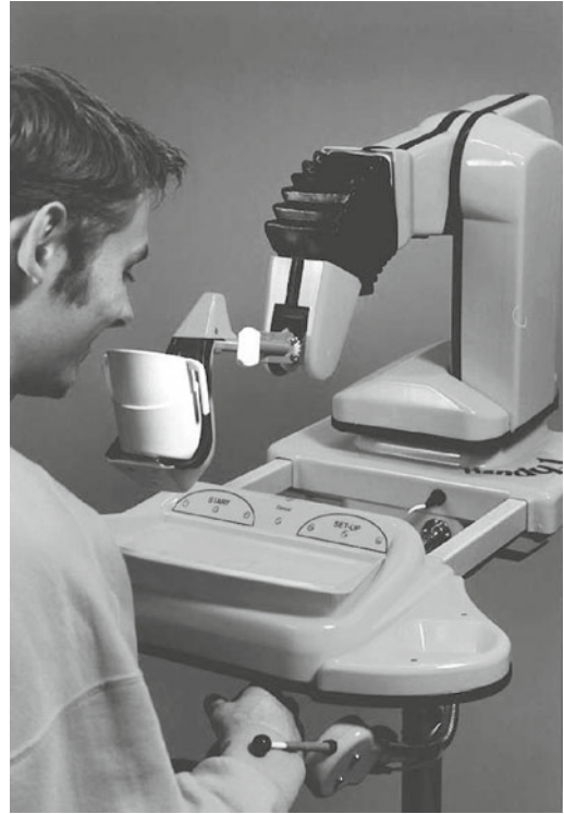
Fig. 6.3 The Handy 1 workstation, intended to help users with eating, drinking, and grooming. First developed by Mike Topping at Staffordshire University (Reprinted with permission from: Topping M. Flexibot —a multi-functional general-purpose service robot. Ind Robot 2001;28:395–401. © Emerald Group Publishing Limited; all rights reserved)
