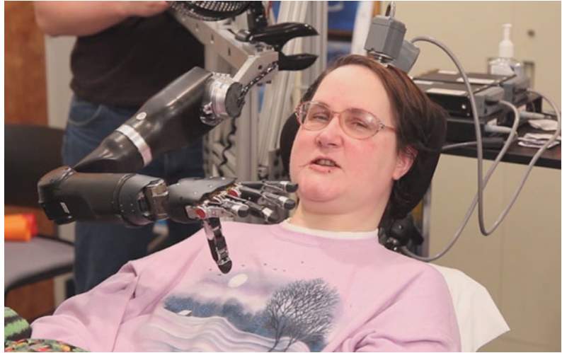
Fig. 6.10 BMI-controlled robotic limbs. Woman with tetraplegia uses modular prosthetic arm to grasp and manipulate objects (photo courtesy of Motorlab, University of Pittsburgh)
