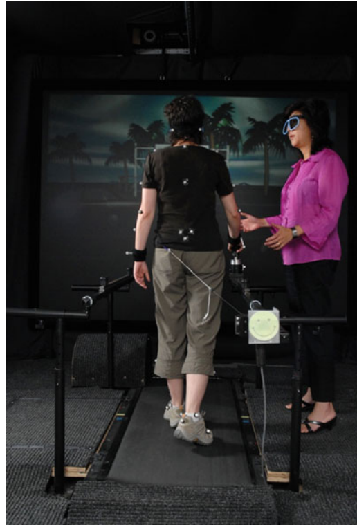
Fig. 20.1 An interactive VR-coupled locomotor system [55] incorporating a self-paced treadmill and dynamic haptics [58] mounted on a six-degree-of-freedom motion platform. Computer-controlled, synchronized animations are rear-projected onto a large screen that can be viewed in 3D with polarized glasses. Such a system can be used to train locomotor adaptation needed to meet demands related to the changing environment (obstruction and surface angle, etc.), tasks (speed requirements, avoiding moving obstacles, dual-tasking, etc.), and cognitive requirements (attention, planning, etc.). Reproduce with permission of Joyce Fung
