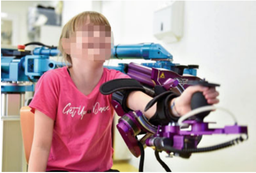
Fig. 14.11 ChARMin. The Children’s Arm Mechatronic Interface (ChARMin) is an upper extremity exoskeleton robot with actuated joints. It was designed to train shoulder, elbow, forearm, wrist, and hand grasping movements of children and adolescents with major upper limb motor impairment. Picture with kind permission from the University Children’s Hospital Zurich
