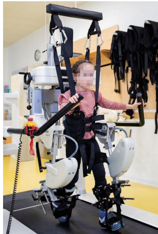
Fig. 14.4 Lokomat. The exoskeleton Lokomat consists of a treadmill, a bodyweight support system and a robotic gait orthosis that can fully guide the leg movements. Newer versions also allow more kinematic freedom, making the device applicable to patients with fewer lower limb impairments. Picture with kind permission from the University Children's Hospital Zurich
