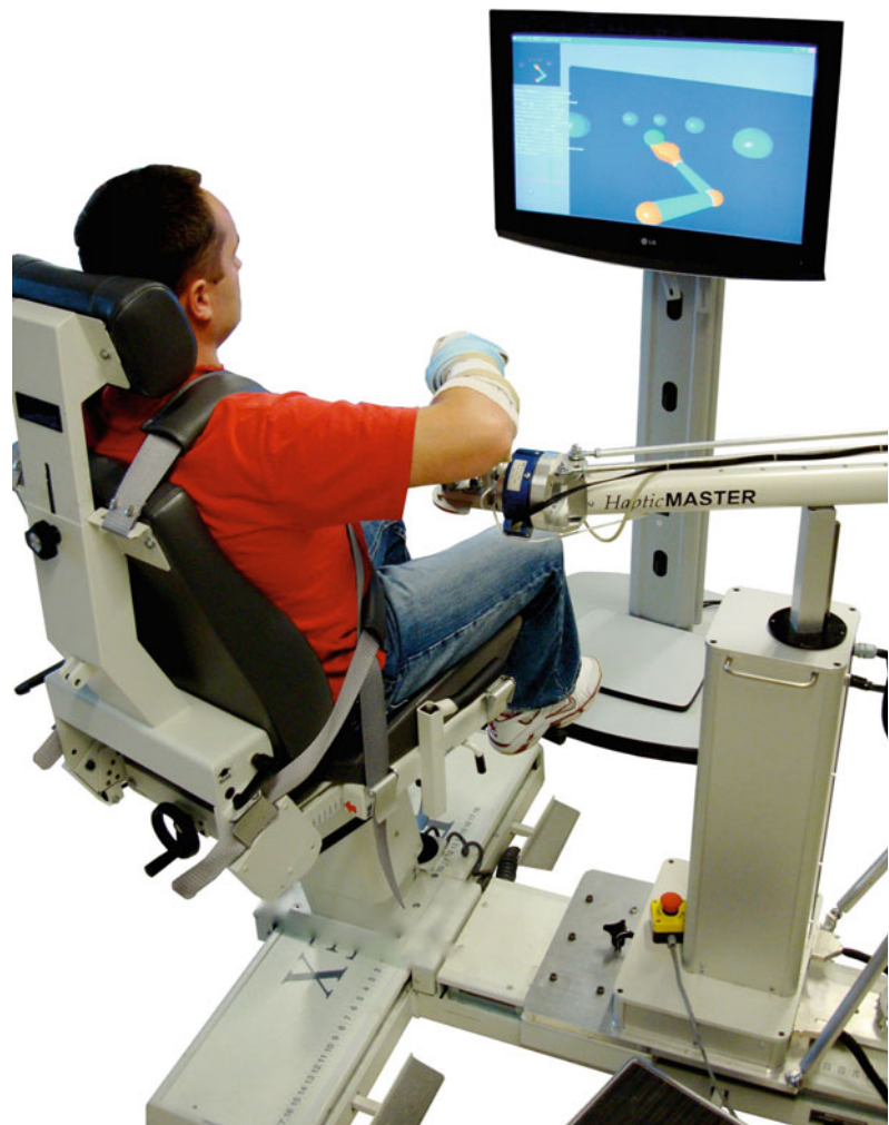
Fig. 5.6 Example of a research participant positioned with the ACT-3D showing the five reaching targets. From Ellis MD, Sukal-Moulton TM, Dewald JP (2009b) Impairment-Based 3-D Robotic Intervention Improves Upper Extremity Work Area in Chronic Stroke: Targeting Abnormal Joint Torque Coupling With Progressive Shoulder Abduction Loading. IEEE Trans Robot 25:549–555; used with permission
