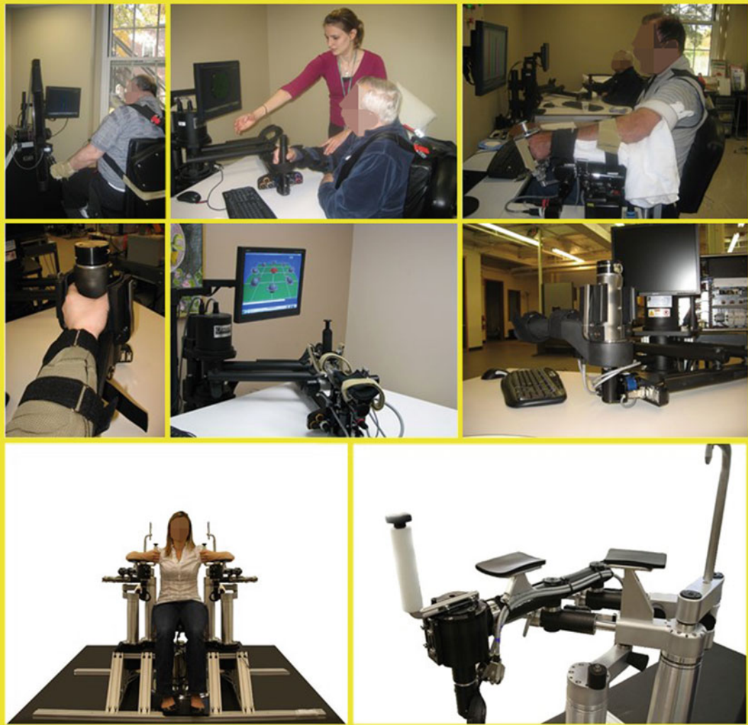
Fig. 26.1 A Gym of Upper Extremity Robots. The top row, left shows a person with chronic stroke working with the anti-gravity shoulder-and-elbow robot. The top row, middle panel shows a person working with the planar shoulder-and-elbow robot. The top row, right panel shows the wrist robot during therapy at the Burke Rehabilitation Hospital. The middle row, left panel shows the hand module for grasp and release. The middle row, middle panel shows reconfigurable robots. The robotic therapy shoulder-and-elbow and wrist modules can operate in stand-alone mode or be integrated into a coordinated functional unit. The middle row, right panel shows the shoulder-and-elbow and hand module integrated into a coordinated functional unit. The bottom row shows an exoskeletal robot with 3 active DOFs designed for psychophysical studies of the shoulder, elbow and wrist. For this exoskeletal robot, the links must be adjusted to the person's limb segments (using laser pointers). Once the arm, forearm, and wrist are properly adjusted, psychophysical experiments can assist or selectively apply perturbation force fields to the shoulder, elbow, and wrist (either flexion/extension or abduction/adduction)
