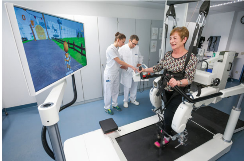
Fig. 13.3 The Lokomat is an active exoskeleton which is operated in conjunction with a moving treadmill
