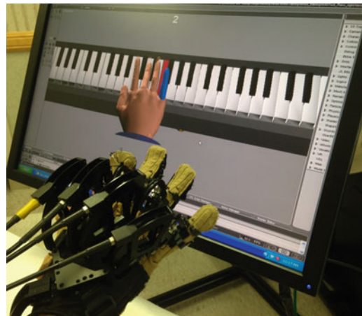
Fig. 20.2 The NJIT-TrackGlove system utilizes a six-degree-of-freedom magnetic tracker, the TrakStar (Ascension Technology Corporation, USA) and a 22-DOF CyberGlove (CyberGlove Systems USA). The simulation pictured also utilizes the CyberGrasp, a cable-actuated robotic exoskeleton. In the pictured simulation, the Virtual Piano Trainer, the magnetic tracker allows the participant to position their hand over the virtual keyboard and the CyberGlove allows them to strike keys with a specific finger. The CyberGrasp can be programmed to provide haptically rendered collisions when keys are pressed or assistance in maintaining extension of non-cued fingers for more impaired subjects [105]
