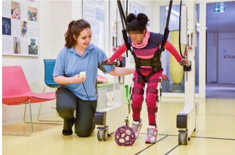
Fig. 14.7 Andago. The Andago allows over-ground bodyweight supported walking on flat surfaces. It enables the therapist to focus more on the child, as the device provides partial bodyweight unloading and prevents falls. Picture with kind permission from the University Children's Hospital Zurich
