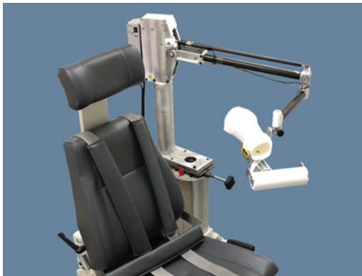
Fig. 5.9 The new PACT-3D is designed to allow safe and efficient use in the clinic and home for stroke upper limb rehabilitation and flexion synergy impairment measures
