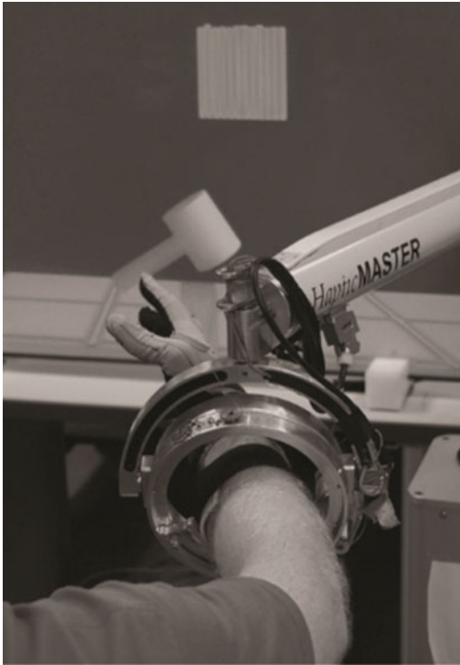
Fig. 20.3 The NJIT-RAVR system utilizes a three-degree-of-freedom robotic (DOF) interface, the Haptic Master (Moog, The Netherlands), three additional passive DOF via a ring-gimbal, and a 22-DOF CyberGlove (CyberGlove Systems USA). The Haptic Master is used to provide haptic rendering of virtual workspaces and add global forces such as gravity to the virtual environments. The ring-gimbal allows for normal positioning of the hand during simulated tasks and the CyberGlove collects data related to finger position. These interfaces are integrated with a suite of complex, virtually simulated tasks to allow for task-based sensorimotor training for persons with upper extremity hemiparesis [67]
