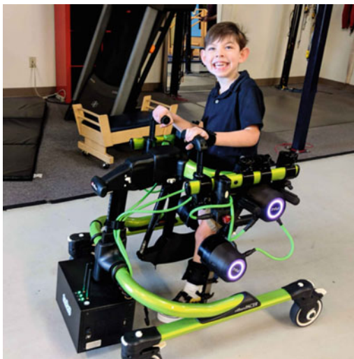
Fig. 14.5 Trexo. The mobile robotic gait training device Trexo consists of a wheeled frame including a battery, robotic legs, and a tablet to control it. A seat, arm, and chest prompts can be used to support the weight and remain balanced. Picture with kind permission from Trexo Robotics Inc
