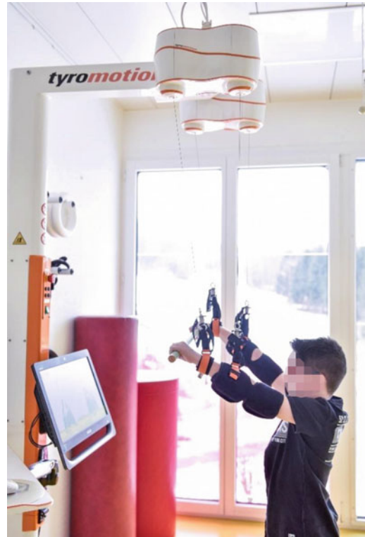
Fig. 14.12 The Diego. The end-effector device Diego provides weight support of the arms and allows both unilateral and bilateral exercises. Picture with kind permission from the University Children’s Hospital Zurich
