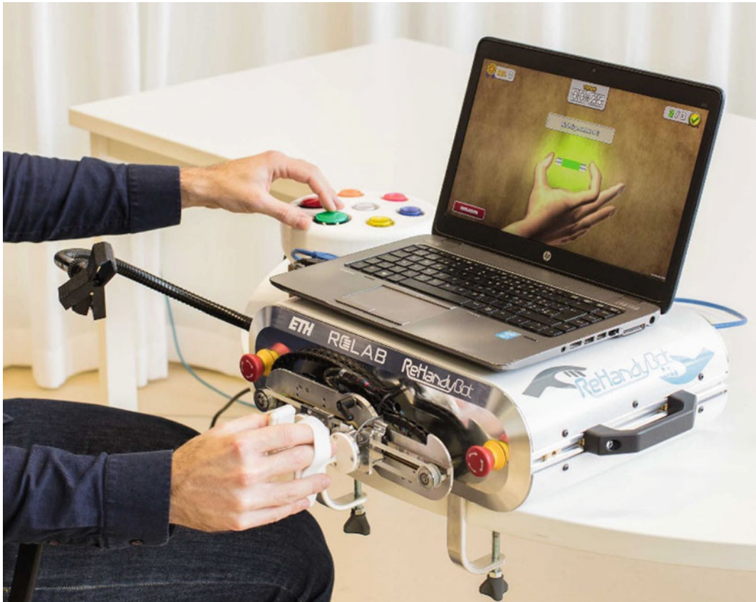
Fig. 25.1 The ReHandyBot (picture: Rehabilitation Engineering Laboratory, ETH Zurich/Stefan Schneller). Fingers and thumb are fixed to separate grippers. Grippers' movement is coupled which allows training hand opening and closing. Moreover, assistive or resistive forces allow haptic feedback and interaction with virtual objects
