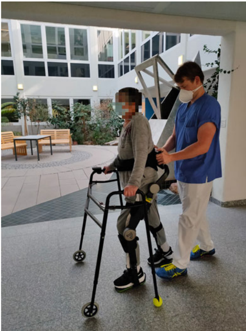
Fig. 13.4 The lightweight ABLE exoskeleton (ABLE Motion, Barcelona, Spain) with actuated knee joints for overground locomotion training [69]
