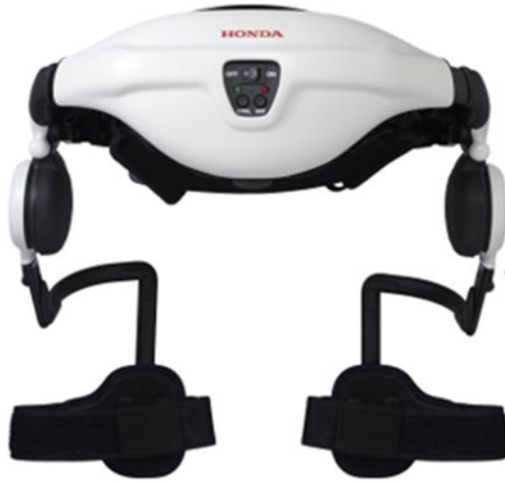
Fig. 30.4 Honda Walking Assist Device (Photo courtesy of Honda Research and Development Company, Ltd.)
