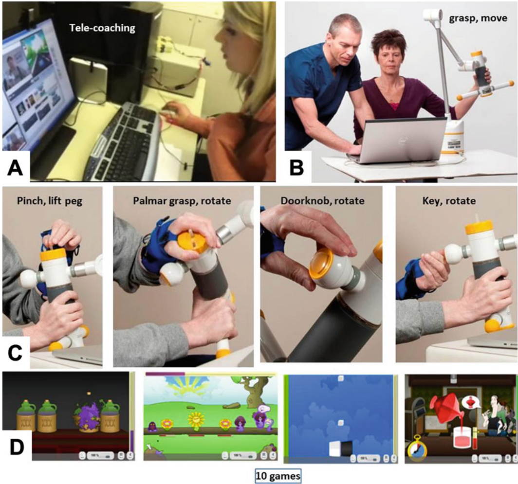
Fig. 23.3 a Tele-coaching of an in-home exercise therapy session using the rehabilitation joystick for computerized exercise (ReJoyce) system; b participant using ReJoyce workstation to play computer games; c movements performed, d selected games
