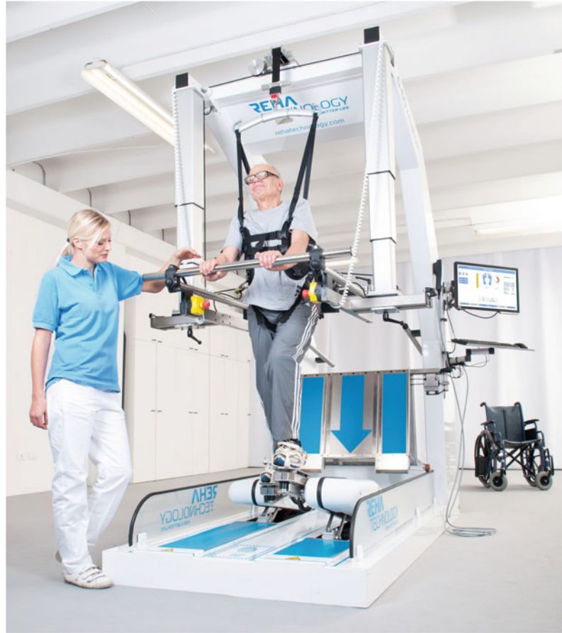
Fig. 13.2 The GEO System assists the patient during gait training using an end-effector-based approach combined with a system for partial unloading of the body weight (Photo courtesy Reha Technology AG, Olten, Switzerland. Used with permission)
