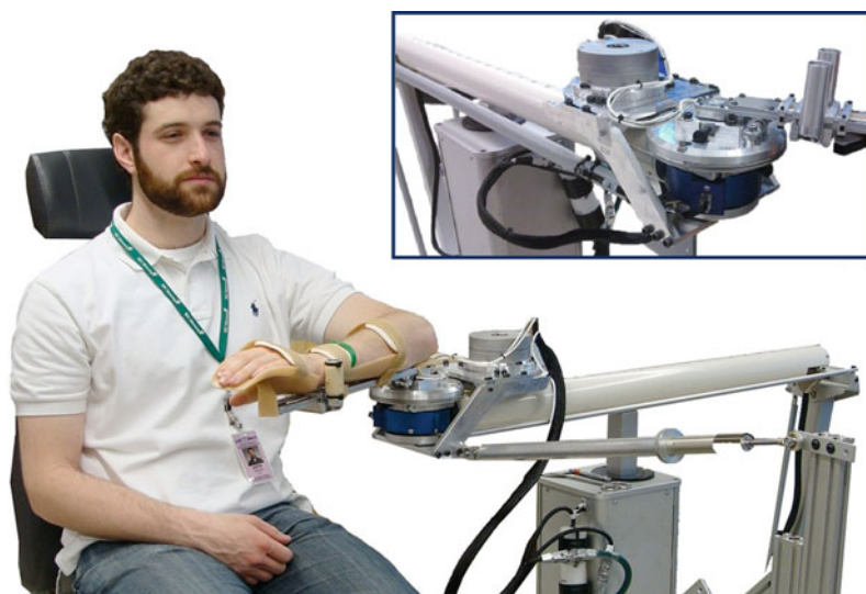
Fig. 5.7 The ACT-2D robotic device allows for single joint perturbations at the elbow combined with adjustable shoulder abduction loading to study the relationship between synergies and abnormal stretch reflex or spasticity following brain injury
