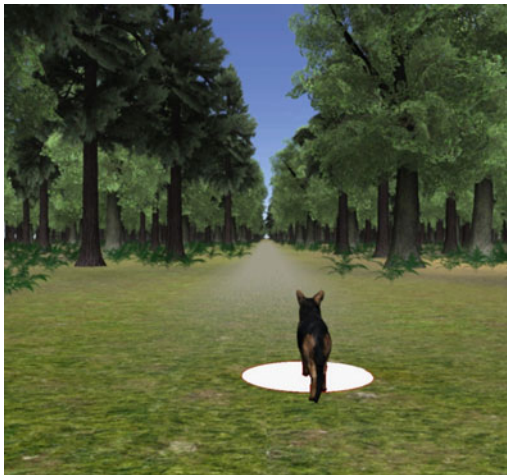
Fig. 10.3 Visual feedback for heart rate control in the Lokomat [21]. The patient's actual effort is shown as a white dot on the screen while the dog represents the desired effort, thus encouraging patients to modify their walking speed. Figure originally from Koenig et al. [21], licensed under CC-BY 2.0
