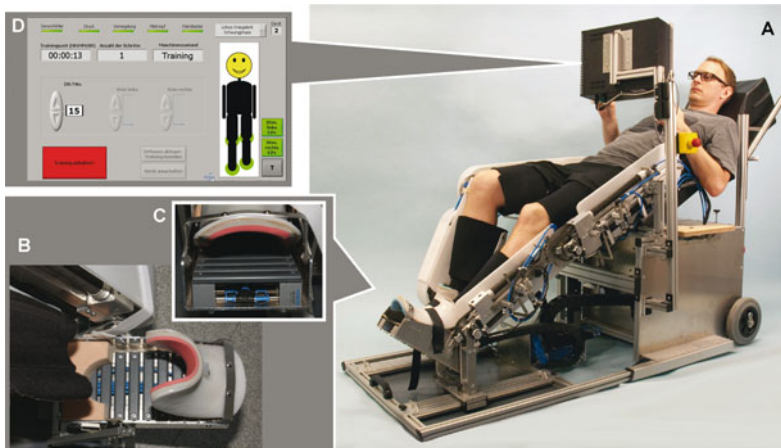
Fig. 13.5 The MoreGait is a pneumatically actuated robot for the training of walking function. The device allows the use at the patient's home: An individual during training (A), top (B), and front (C) view of the mediolateral bars of the stimulative shoe for mechanical stimulation of foot loading afferents, user interface, and feedback screen (D)
