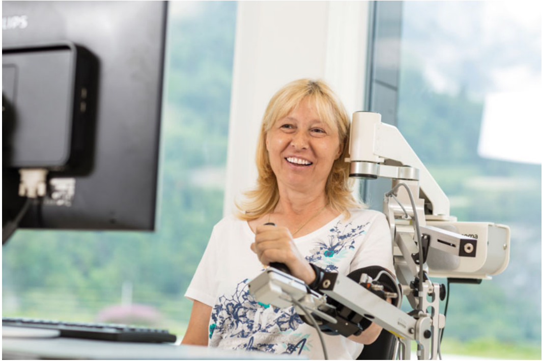
Fig. 28.2 ArmeoSpring, developed by Hocoma AG based on T-WREX, is designed to be more quickly adjustable than T-WREX for easier clinical use (Picture: Hocoma, Switzerland)
