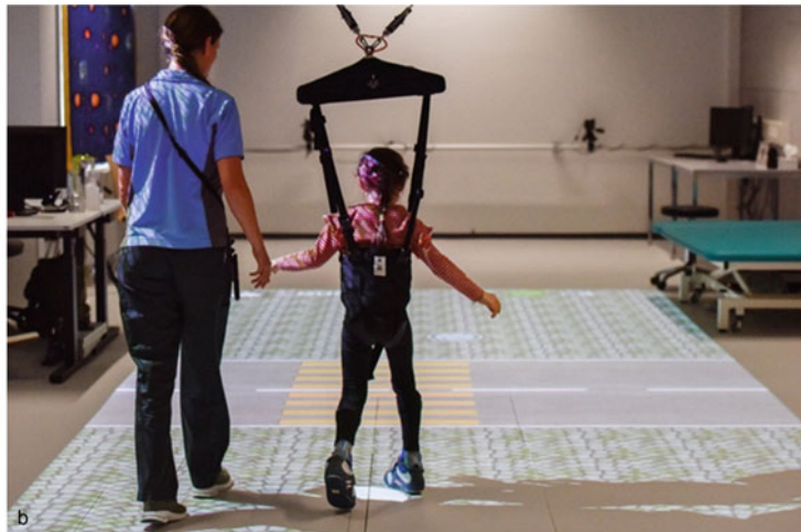
Fig. 14.8 RYSEN. a , The RYSEN allows relatively free walking within the space that is predefined by the system. It has excellent transparency, particularly in the forward-backward direction. It can be used to train various tasks like balancing, stepping over obstacles, walking up or downstairs, standing up, and sitting down. b , RYSEN can be combined with three beamers enabling large floor projections that can provide funny, challenging, and goal-specific exergaming. Picture with kind permission from the University Children's Hospital Zurich
