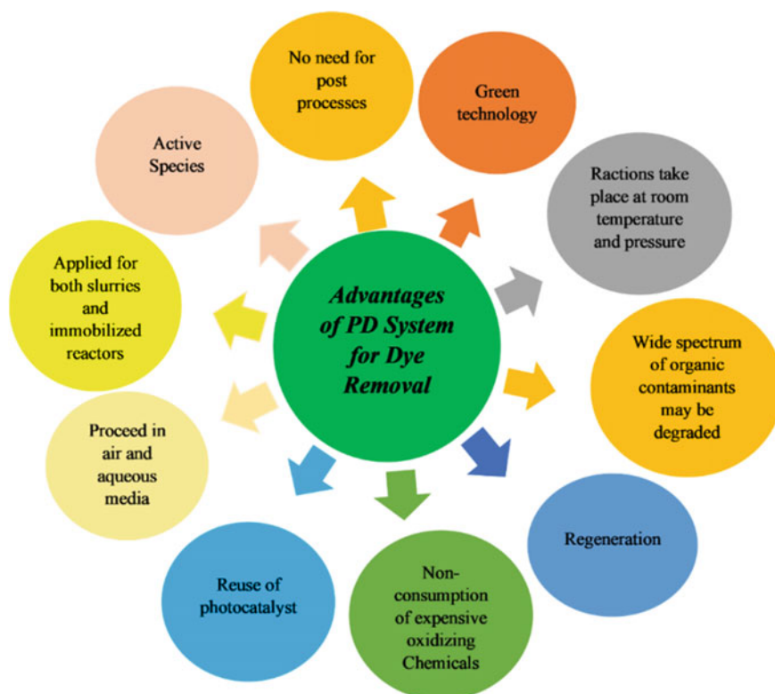
Fig. 2.1 Key advantages and efficiency of PD technologies for dye removal
