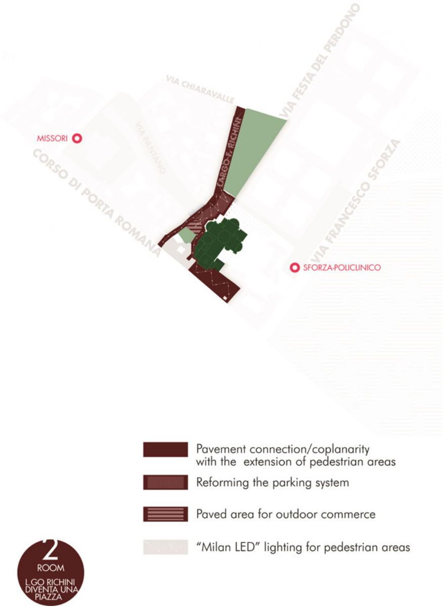
Fig. 5.3 Sforza-Policlinico, the campus station and the new public square in Largo Richini. The diagram identifies the priority actions for reorganising the public space that surrounds the asilica di San Nazaro in Brolo, proposing the redesign of draining paving and a reduction in areas accessible to motorised vehicles to promote pedestrian uses and connections
