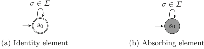
Fig. 4. Finite state automata acting as identity element and absorbing element for the automata cross-product operation.
