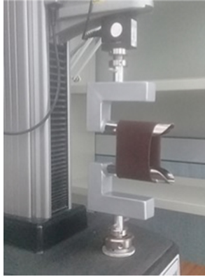
Fig. 1. Customized grips for Lloyd S5 testing machine.
