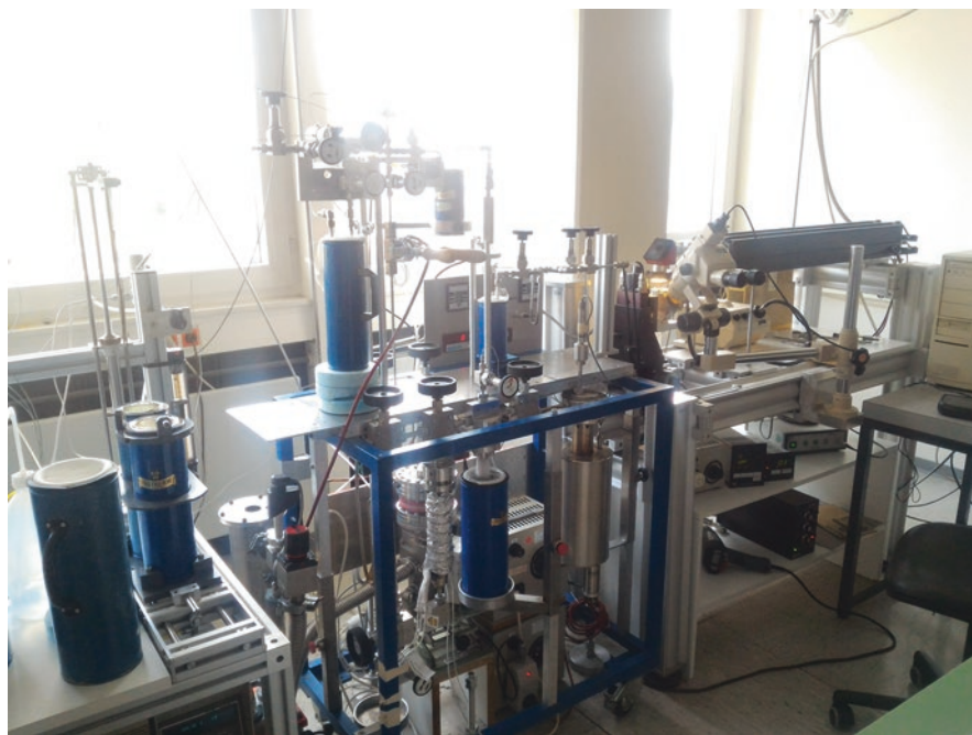
Fig. 9.4 An example of gas extraction and purification line. (Source: Geowissenschaftliches Zentrum, Abteilung Geochemie, Georg-August-Universität, Göttingen, Germany. Photo courtesy by R.S. Iovine)
