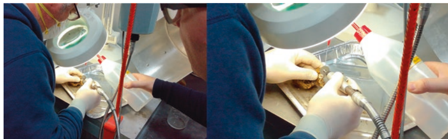
Fig. 9.3 Cutting of a tooth using a dental drill equipped with a diamond-coated saw. (Source: Radiogenic Isotope Laboratory, National Institute of Geophysics and Volcanology, Section of Naples Osservatorio Vesuviano, Naples, Italy (Photo by M. D'Antonio))
