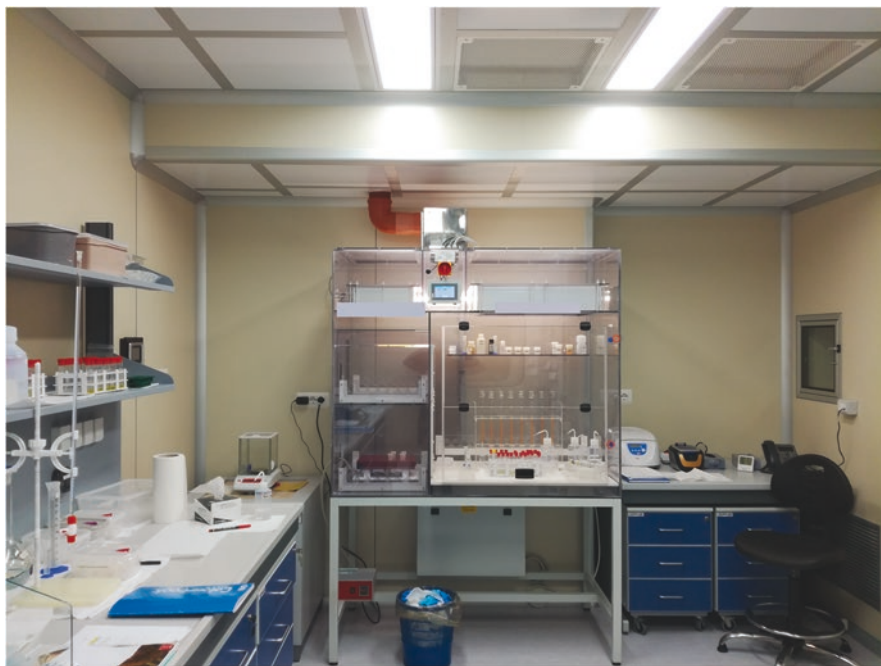
Fig. 9.1 ISO 6 class clean room. Notice the High Efficiency Particulate Air (HEPA) filters on the ceiling from which clean air enters the room and, in the background, a Perspex laminar flow hood equipped with two HEPA filters located on top, to achieve ISO 5 class. (Source: Clean Room, Department of Earth, Environmental and Resources Sciences (DiSTAR), University Federico II, Naples, Italy. Photo by M. D'Antonio)
