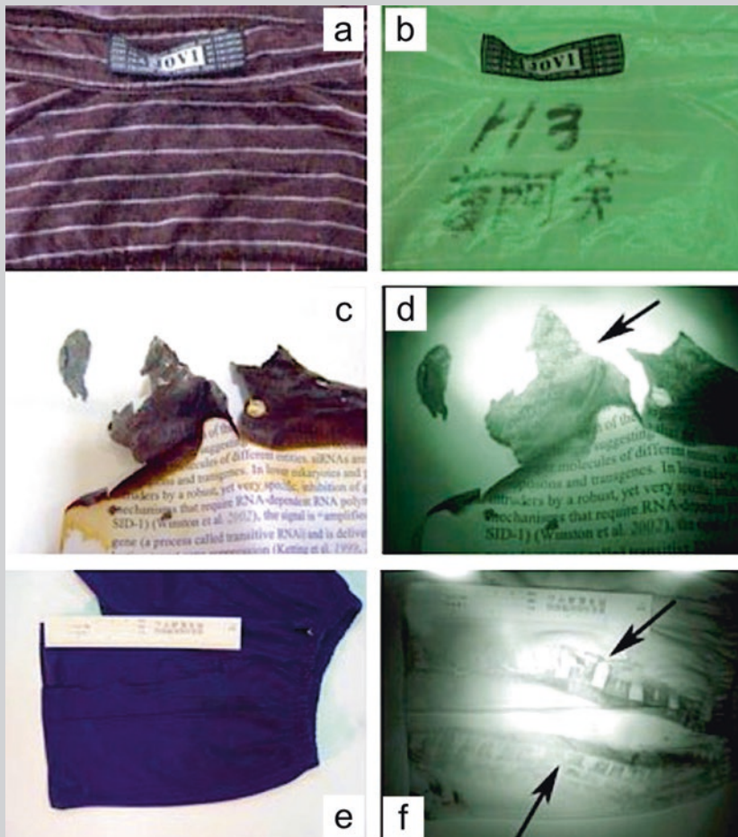
Fig. 4.20 A section of underpants viewed in visible light (a) and using the infrared portion of the spectrum (b); in the latter case, the stripes are suppressed, and a written inscription enhanced. No text is visible in the burnt portion of a document (c), yet it is apparent when using IR imaging (d). A blue pair of shorts reveals nothing out of the ordinary in visible light (e), yet an apparent imprint of a rubber tire is visualized when viewing the object in IR (f). (Modified after Lin et al. 2007).
