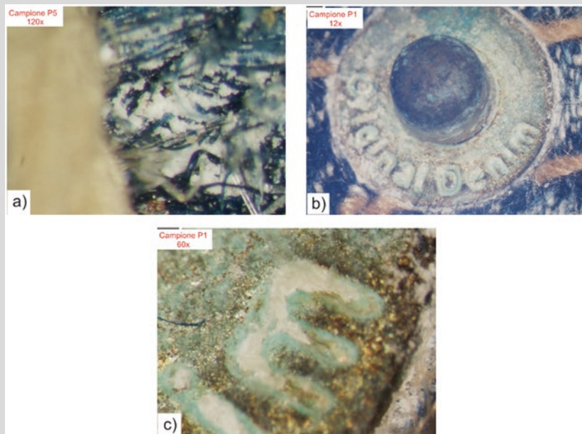
Fig. 1.10 Victim's jeans observed under a stereoscopic microscope: (a) White micro-crystals near the hems of the pockets (120 \times ); (b) Metal rivet with white micro-crystals along the rivet circumference and in the engraved inscriptions (12 \times ); (c) Particular of white micro-crystalline patina inside the engraved letter (60 \times ). (Courtesy of SCARLabs srl, Caserta, Italy)
