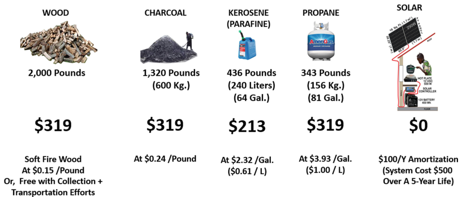
Fig. 5. Annual fuel needed to cook three meals per day for a family of four in Kenya (2022)
