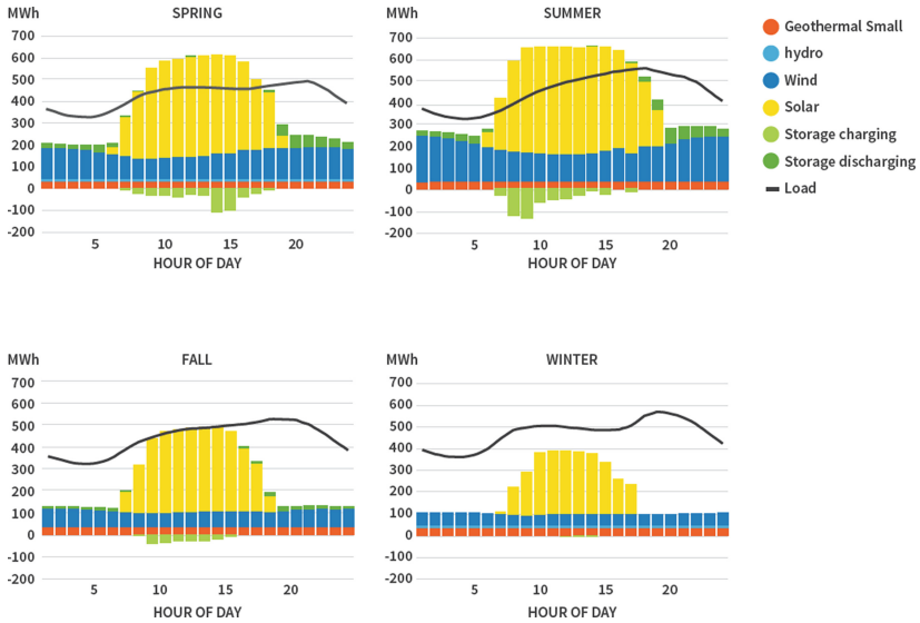
Fig. 2. Seasonal load profile and contracted resources for 2025. For each season of the year 2025, this plot shows the average hourly match between our forecasted load and currently contracted resources, as well as hypothetical energy storage dispatch. This puts us on track to be 64% renewable on a time-coincident basis in 2025 if we were to take no further actions.
