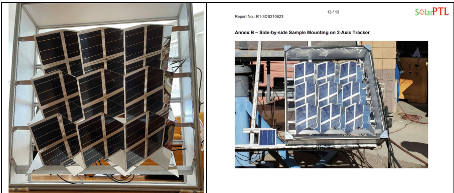
Fig. 2. (A) 3D Solar “dual hybrid” prototype module, containing 9 PV cells. Cells are located on the upper left, with reflectors on right and below. (B) Side-by-Side testing setup on tracker at Solar PTL. Individual “control” cell on lower left; 3D Solar prototype on right.
