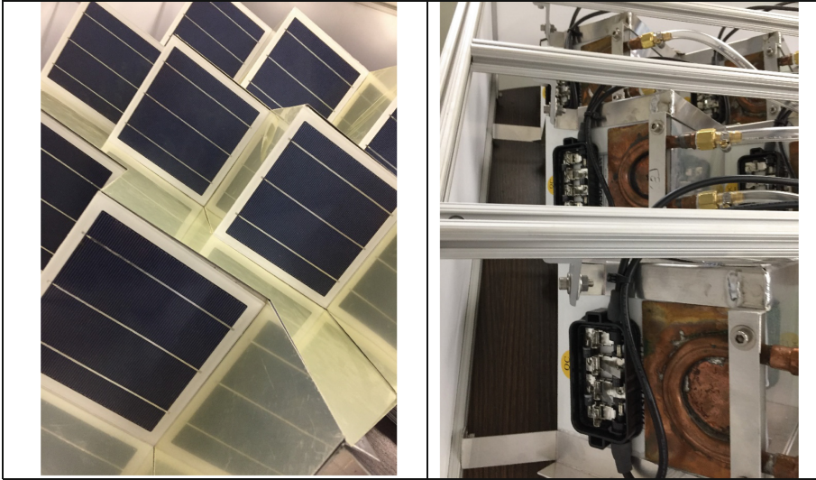
Fig. 1. (A) Close up of multiple cell reflector pairings. Cell is placed at a 90° angle to each reflector. The reflectors have a protective coating—giving them a dull yellow appearance. (B) Close up of back side of a laminated cell. Shows modified (squashed) copper fin-tube in contact with ~1/2 of the back of each cell
