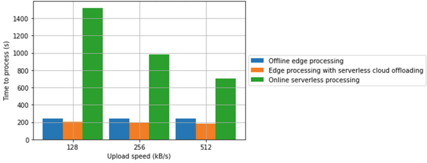
Fig. 3. Dependency between the basecalling execution time and upload speed for various strategies of data processing for highest power mode of Jetson Xavier NX (offline edge processing vs. edge with cloud offloading vs. online serverless processing).
