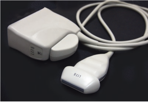
Fig. 4.6 Linear array transducer. High variable-frequency (6.0–18.0 MHz) ultrasound (HVFUS) linear array transducers have a higher resolution but lower penetration than convex transducers and are used for superficial applications
