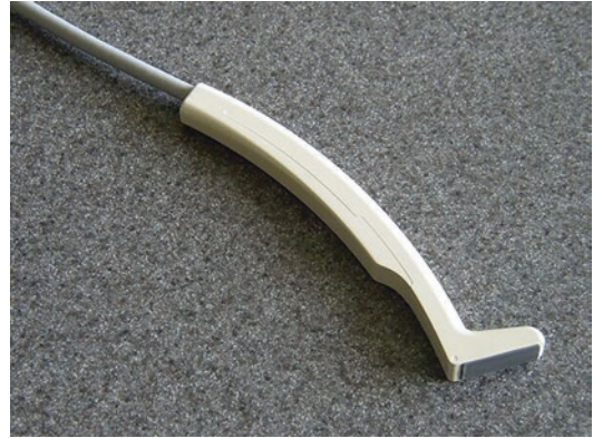
Fig. 4.7 “Hockey stick” transducer. Versatile multifrequency (up to 13 MHz) linear compact, hockey stick-shape transducer, with a high Doppler and color flow sensitivity. The “hockey stick” shape allows complete contact with the skin surface, reducing scattering artifacts, making it a good choice for small superficial structures, including vascular imaging
