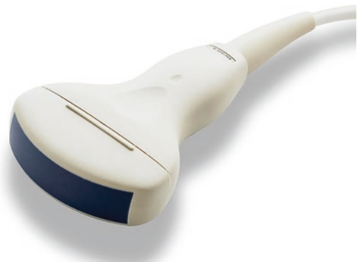
Fig. 4.5 Convex array transducer. Low-frequency (up to 6 MHz) convex-shaped transducer. Convex transducers are used for imaging deeper structures like abdominal organs due to their higher penetration, although at the price of a lower resolution
