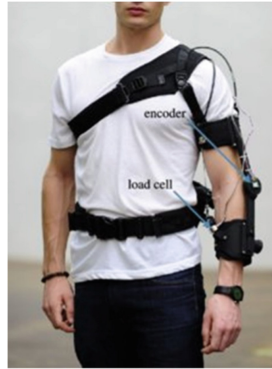
Fig. 1. Example of upper-limb assistance exoskeleton. [4]
