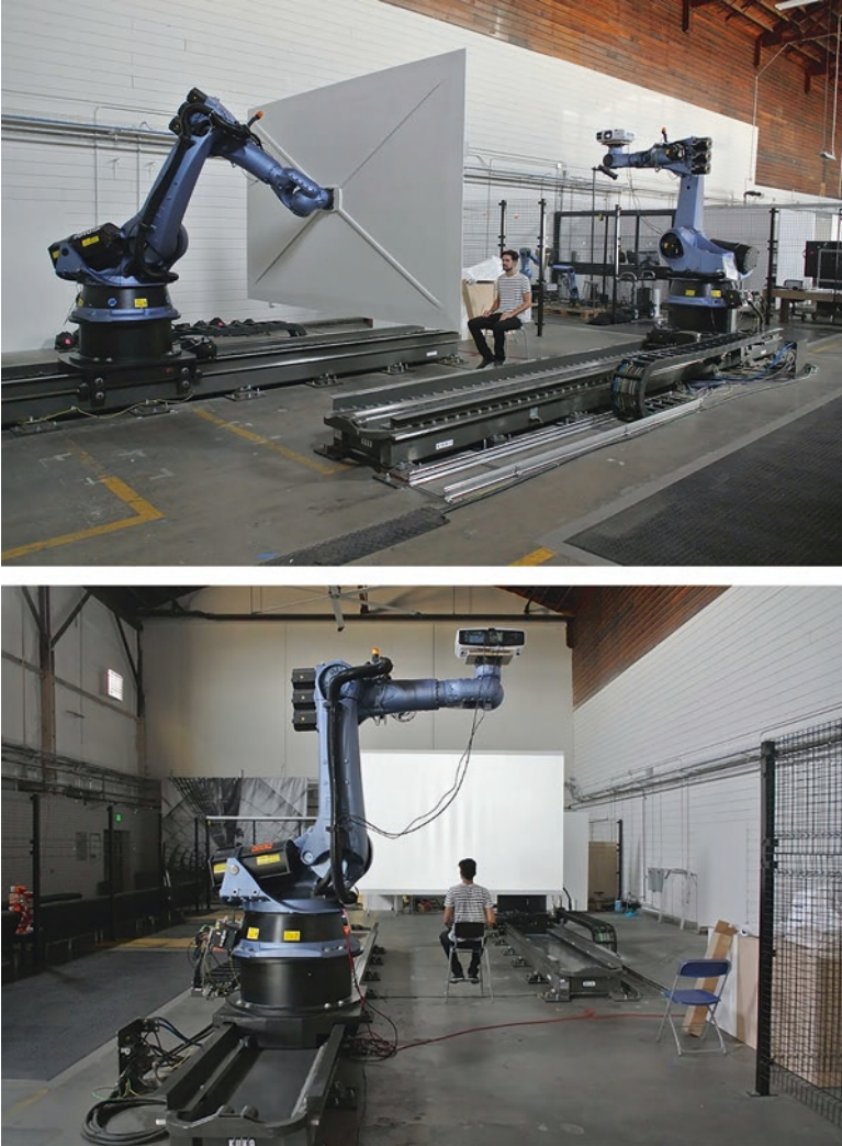
Fig. 12.4 Apparatus for measuring pattern visibility on a large spatial scale. Two industrial robots carried a projector and a screen in a study designed to measure boundaries of visibility on the scale of architectural design. The two panels show a side view and a back view of a person facing the screen
