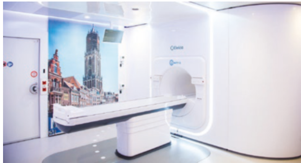
Fig. 6.3 Clinically used Elekta Unity MRI-Linac at the UMC Utrecht hospital, Utrecht, The Netherlands
