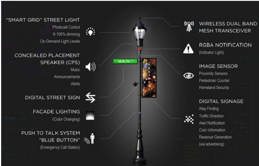
Fig. 2. Public smart lighting [26].
