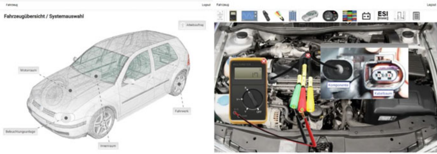
Fig. 8.1 Computer simulation for car mechatronics; Left: Overview of car systems; Right: Resistance measurement of the exhaust gas recirculation valve with a multimeter
