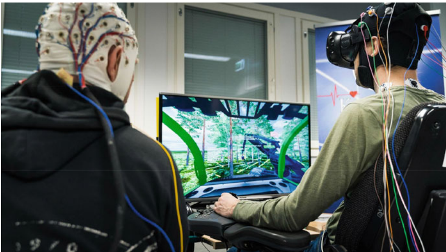
Fig. 7.1 Illustration of the research situation while testing the equipment. The student sat on the right (operating the simulator) and the instructor on the left, and both wore the EEG caps
