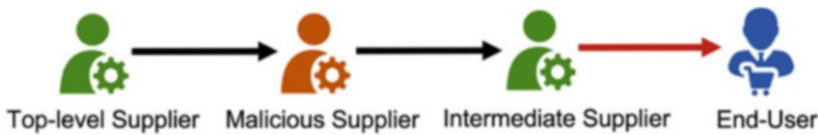
Fig. 1.2 Typical supply chain networks involving nodes and links: A node represents the product suppliers. A link represents the cyber, physical, or logical dependencies of one supplier (or end-buyer) on the other suppliers. The product of an intermediate supplier relies on the transportation and the integration of the products from top-level suppliers. Potential supply-chain attacks may occur both at individual nodes (illustrated by the red color malicious node), supplier links (illustrated by the red color link between the intermediate supplier and end-user), or a combination of the two
