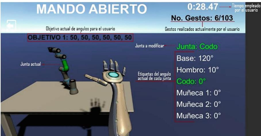
Fig. 3. Visual interface during the tasks execution. Selected joint is highlighted with green. All the time the current and objective values are shown.
