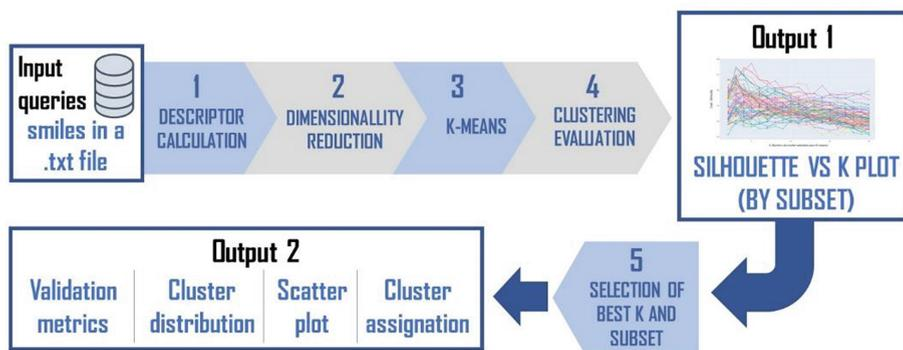
**Fig. 2.** A graphical summary of the RaPCA clustering method, combining feature bagging, principal component analysis and k-means optimization.
