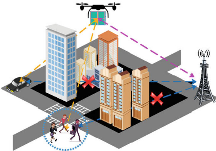
Fig. 6.1 RIS-assisted UAV communication
