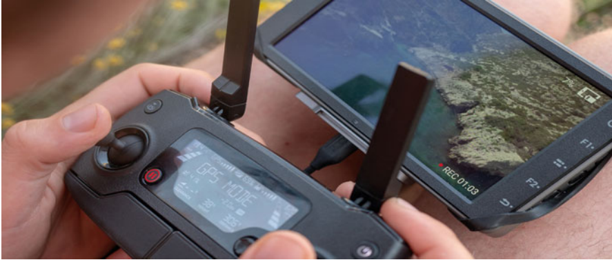
Fig. 13.7 The controller communicates with the drone’s onboard throttle receiver
