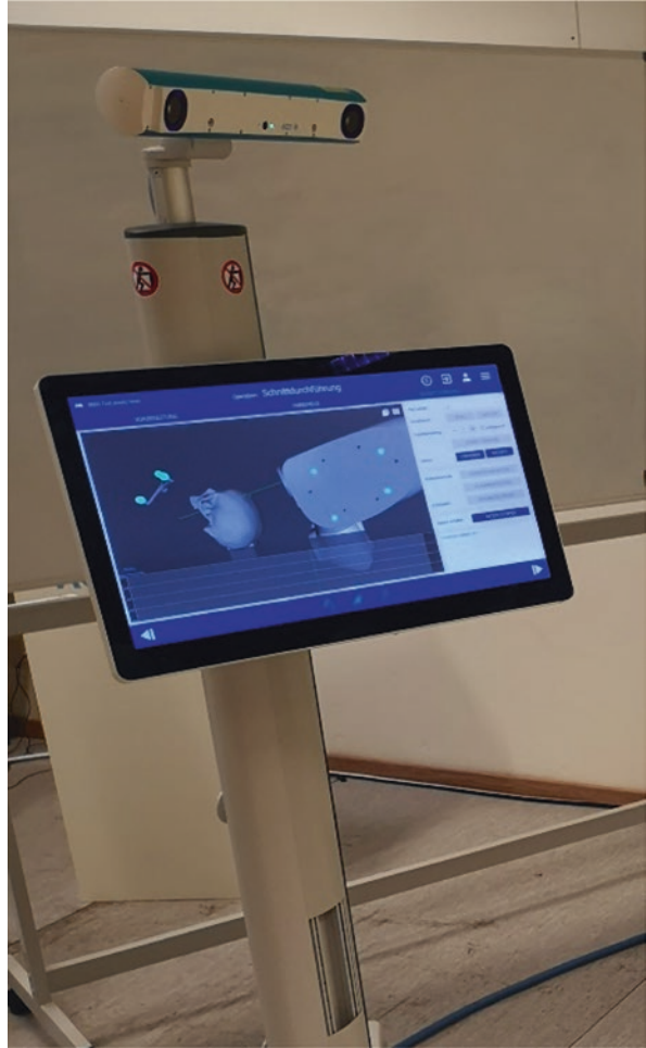
Fig. 14.1 Optical navigation system with two tracking cameras allowing exact procedures
