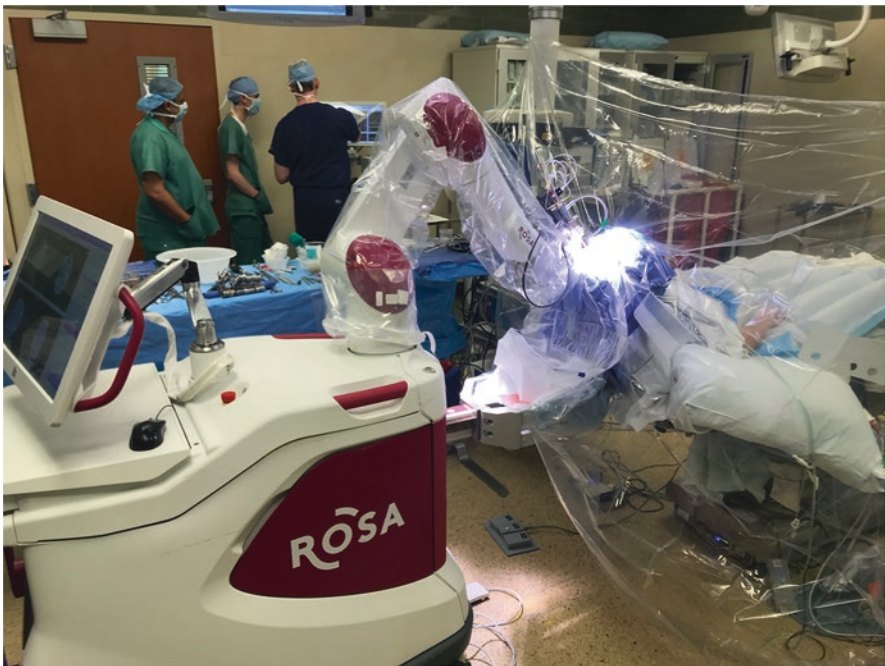
Fig. 5.1 Typical operating setup. The ROSA is positioned in-line with the patient, whose head is elevated to the maximum height possible for attachment of the Leksell frame to the ROSA. A clear operative drape is used to facilitate monitoring of the patient during the “awake” portions of the case. Figure reproduced from Faraji et al. [4]
