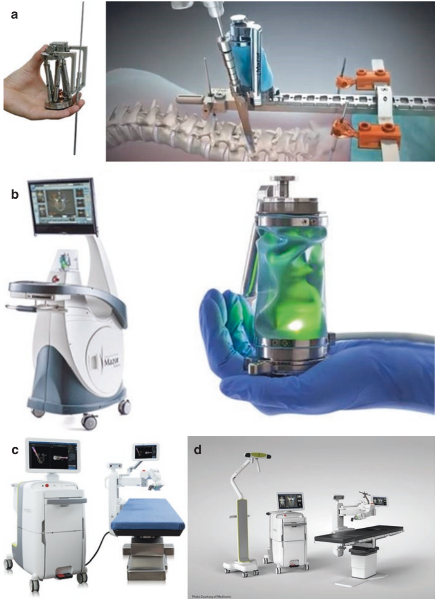
Fig. 16.2 (a) Medtronic SpineAssist robotic system. Image provided courtesy of Medtronic. (b) Medtronic Renaissance spine robotic system. Image provided courtesy of Medtronic. (c) Medtronic Mazor X spine robotic system. Image provided courtesy of Medtronic. (d) Medtronic Mazor X Stealth Edition robotic system. Image provided courtesy of Medtronic
