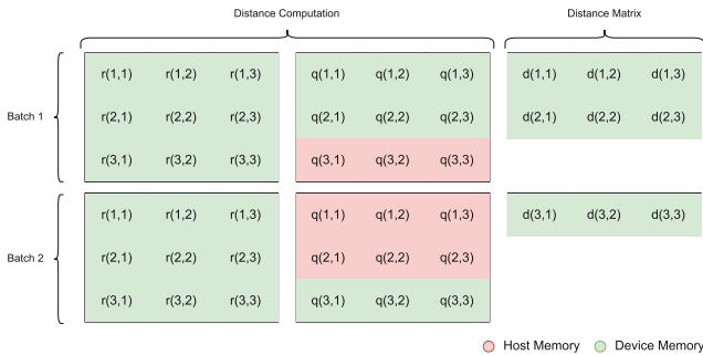
Fig. 1. Exemplary distance computation of three-dimensional points using Q -batch with a batch size of 2 where r(i, \cdot) is a point in the reference set, q(j, \cdot) is a point in the query set and d(j, i) refers to the distance from point q(j, \cdot) to r(i, \cdot) .
