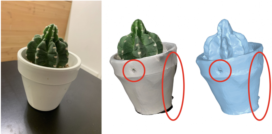
Fig. 5. Example of reconstruction on a reflective surface
