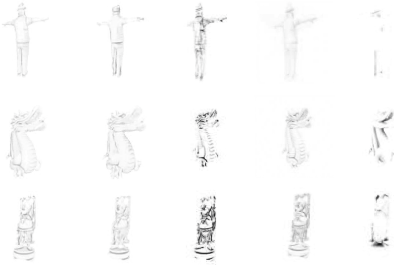
Fig. 6. Qualitative comparison: the first column represents the ground truth images with AO only, the second column represents our result, the third column HBAO [7], and the last two columns represent NNAO [13] and VAO [8].
