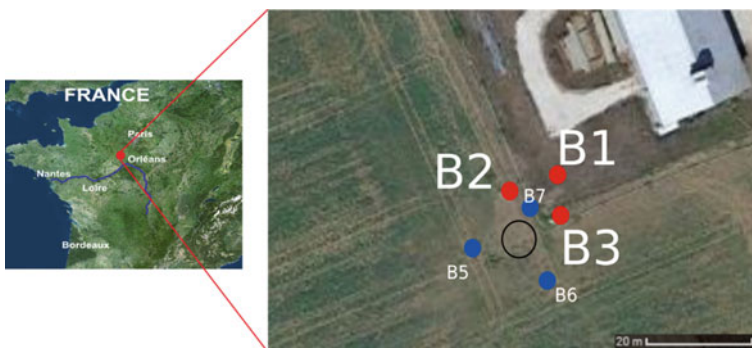
Fig. 19.1 Localization of the O-ZNS site and its organization with the well (black circle) and the six boreholes (in red for the ones from 2017 and blue for the most recent ones from 2020) used for this study
