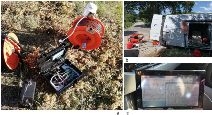
Fig. 16.12 New DERT device system. Receiver (a) and transmitter (b) units are physically separated. Current and potential signal measured in real-time (c)
