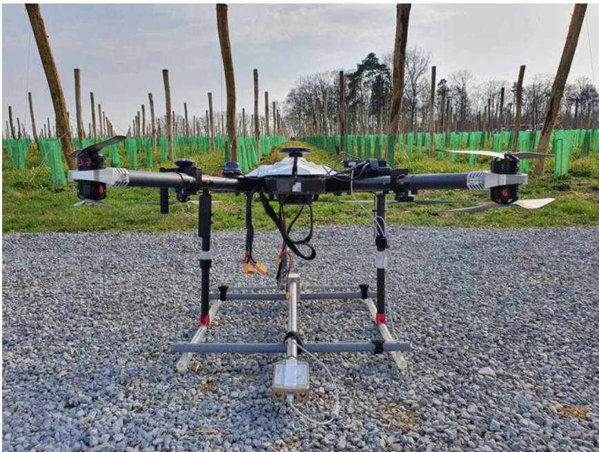
Fig. 17.6 Half-wave dipole antenna and radar mounted on the drone
