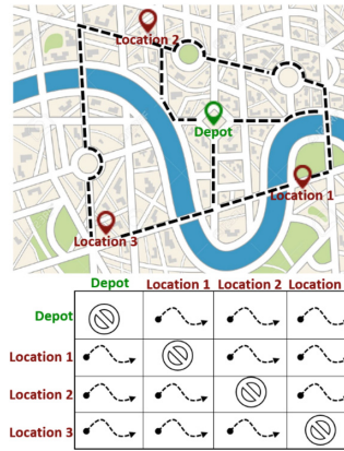
Fig. 2. Path Matrix stores paths computed by A* based on road maps. Paths are calculated for all pairs of locations to be visited, including the depot.
