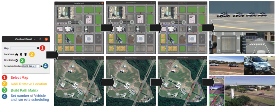
Fig. 4. Route Scheduling. This process shows the flow of our route scheduling system: 1) Select a road map; 2) Set depot and desired locations on the map; 3) Build complete graph and path matrix; 4) Schedule routes for each vehicle using a system algorithm; 5) Send routes to cars.
