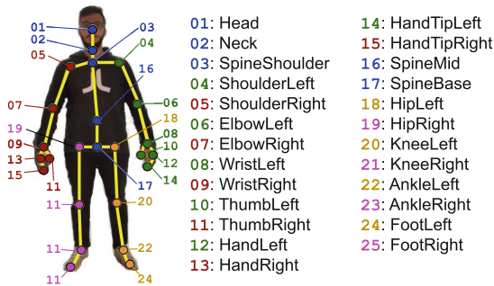
Fig. 1. The 25 skeletal joints extracted by Microsoft Kinect, divided into five main body parts – blue: torso, red: left hand, green: right hand, magenta: left leg, orange: right leg. (Color figure online)
