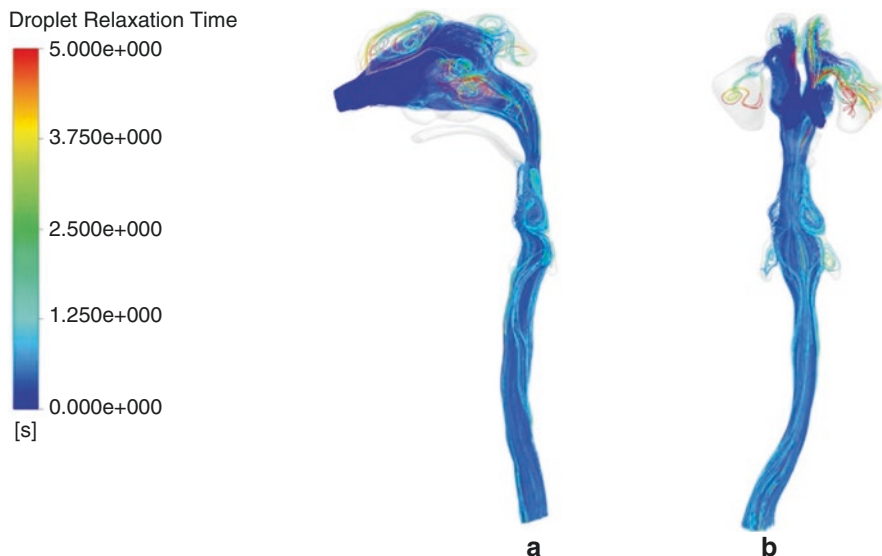
Fig. 6.4 Droplet relaxation contour with average density at 5\ \mu\text{m} , and 6\ \text{L/min} for Group A. (a) Anterior droplet relaxation time tracking. (b) Posterior droplet relaxation time tracking
