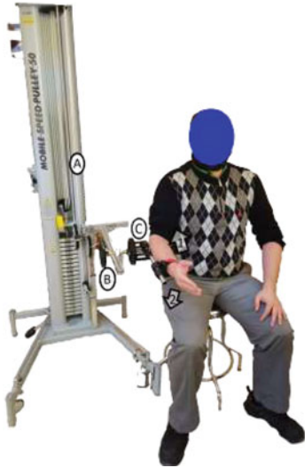
(a) Elbow (1)flexion/(2)extension measurement setup.
