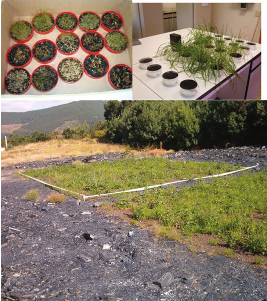
Fig. 5 Images of plants growing on different kinds of waste materials treated with sorbents and by-products in the laboratory (above), and an example of test areas corresponding to restoration tasks performed in a mine spoil area (below) (original from authors, not previously published)
