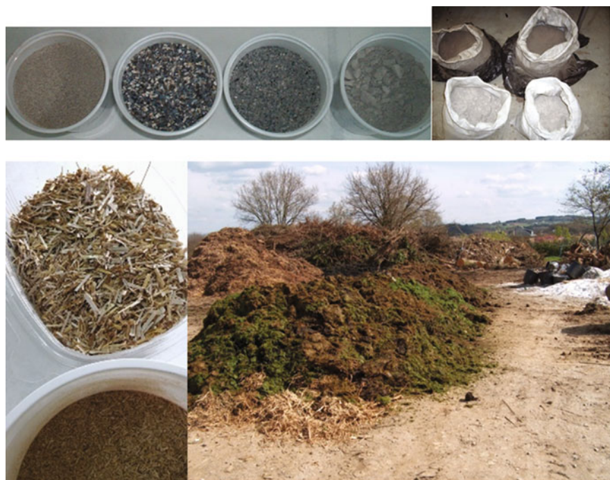
Fig. 4 Images of sorbent materials and by-products used to be mixed with sewage sludge and other wastes containing emerging pollutants, including by-products from mussel shell processing (above), individual vegetable remains and mixtures of them (below) (original from authors, not previously published)
