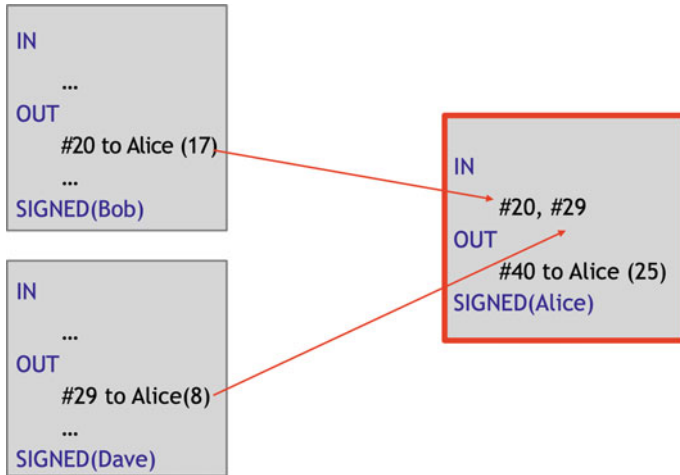
Fig. 7 Bitcoin transaction consolidation: an owner can create a transaction to consolidate the funds from many UTXOs he or she owns
