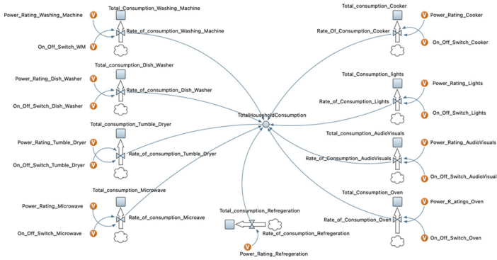
Fig. 2. Anylogic model of the nine HH appliances.
