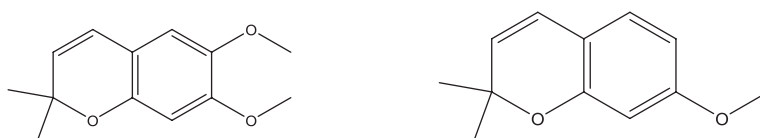
Precocene II (6,7-dimethoxy-2,2-dimethylchromene) Precocene I (7-methoxy-2,2-dimethylchromene)
