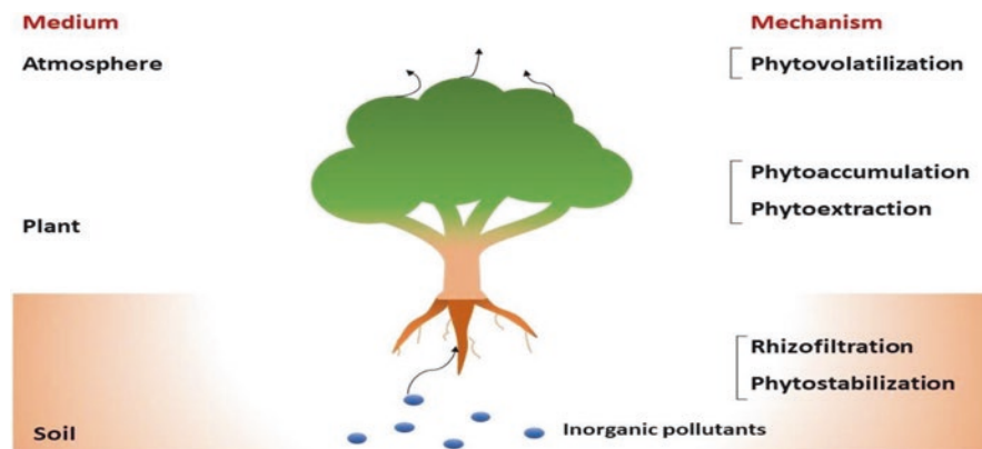
Fig. 3.5 Mechanisms of phytoremediation of inorganic pollutant elements (heavy metals) in soil-plant-atmosphere continuum
