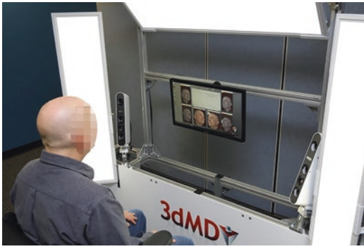
Fig. 2.28 Imaging acquisition with the 3dMDface System. (Courtesy of 3dMD LLC, Atlanta, GA, USA; with permission. ©2021 3dMD. All rights reserved)
