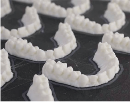
Fig. 4.20 Dental models printed in FDM technology
