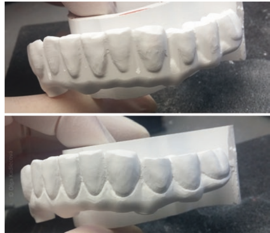
Fig. 5.23 An example of unmilled areas around the gingival margin and interproximal (top) and these areas are manually refined by a dental technician before sintering (bottom picture). (Source: Olga Kadlecová, dental CAD/CAM technician)
