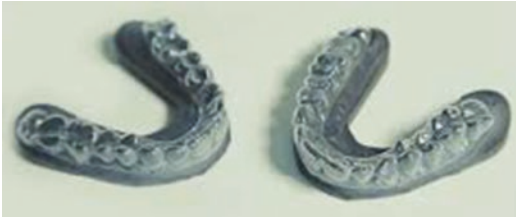
Fig. 4.18 Aligner dental models printed in MJF technology. (Source: HP Inc)
