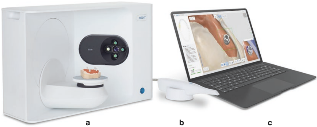
Fig. 2.1 (a) A tabletop scanner scans dental models of patients, and (b) an intraoral scanner directly scans patient's teeth. (c) Both tabletop and intraoral scanner need a computer software for data analysis and storage
