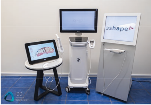
Fig. 5.4 An example of intraoral scanners integrated with mobile computers/carts. Left to right: iTero Element 5D Plus (Align Technology), CEREC Primescan (Dentsply Sirona), TRIOS 3 (3Shape). (Source: Institute of Digital Dentistry, Wellington, New Zealand)
