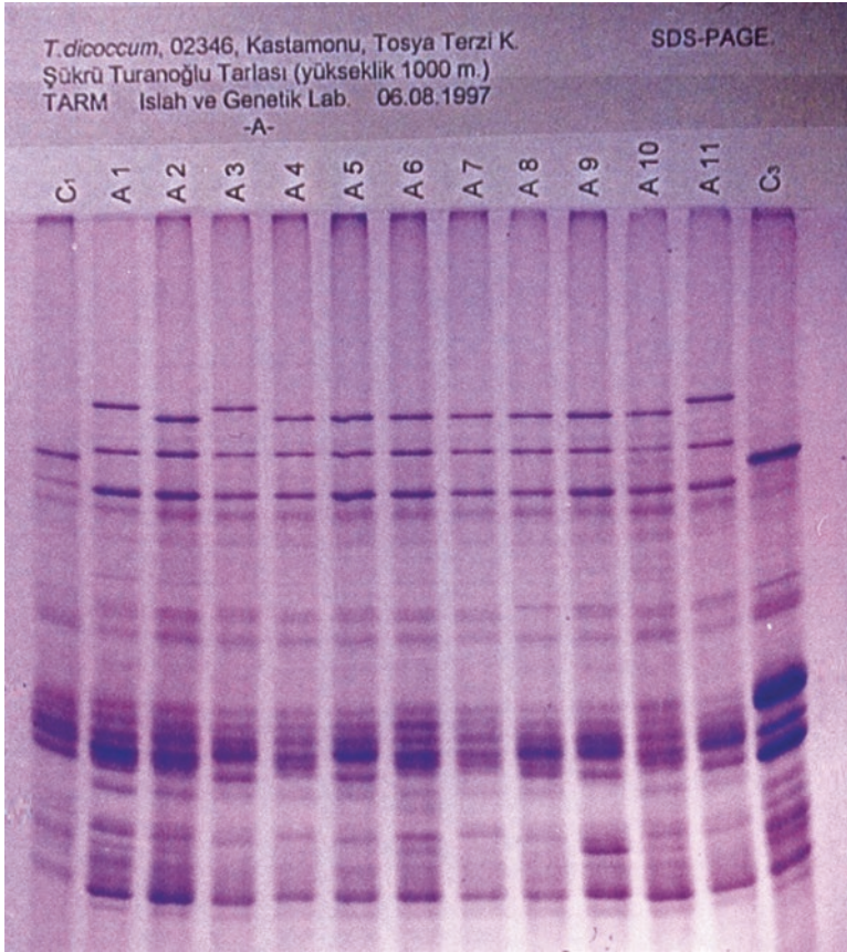
Fig. 4.6 HMW glutenin subunits screened by SDS-PAGE method in Turkish emmer wheat population from Sinop province (Source: Özbek, 1998)
