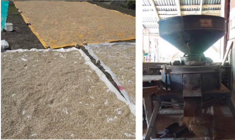
Fig. 7.4 (a) The wheat is dried for 4–5 hours to be slightly moist (left) (HM Yaman) (b) Separation of milled einkorn, by the electrical stone mill, into parts of chaff, dehulled, and broken grains in Kastamonu, İhsangazi (right) (HM Yaman)
