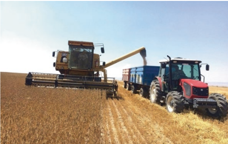
Fig. 4.13 After harvesting, the harvester separated seed grains from their chaffs, and it is evacuating the seed grains into a trailer. (Photo by E.M. Demircan in 2017 with permission)
