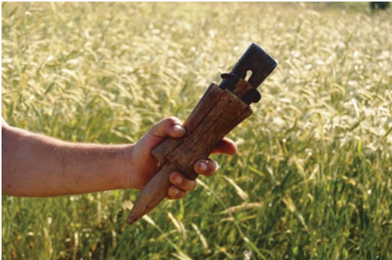
Fig. 4.8 An apparatus used to sharpen the reap hook. (Photo taken in 2017 by Özbek with permission)
