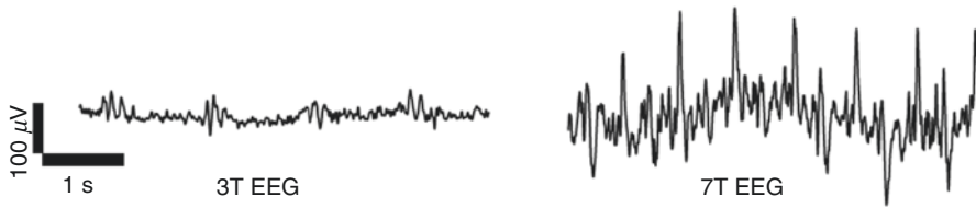
Fig. 11.6 Pulse artifact (PA) amplitude increases substantially at the high magnetic field. An example EEG trace recorded at 3 T vs. a trace recorded at 7 T is shown. The BCG corresponds to the large peaks locked to the cardiac cycle; the amplitude of this noise is greatly increased in the 7 T recording
