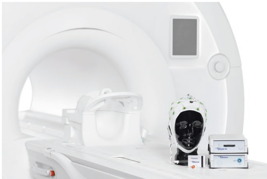
Fig. 7.1 Example of commercial EEG–fMRI instrumentation showing (a) electrode cap, (b) connector box containing current-limiting resistors, (c) battery power pack and (d) 32-channel EEG amplifier/digitiser. This instrumentation is sited adjacent to the scanner bore and transmits data to a receiver outside the Faraday shield via fibre optic links
