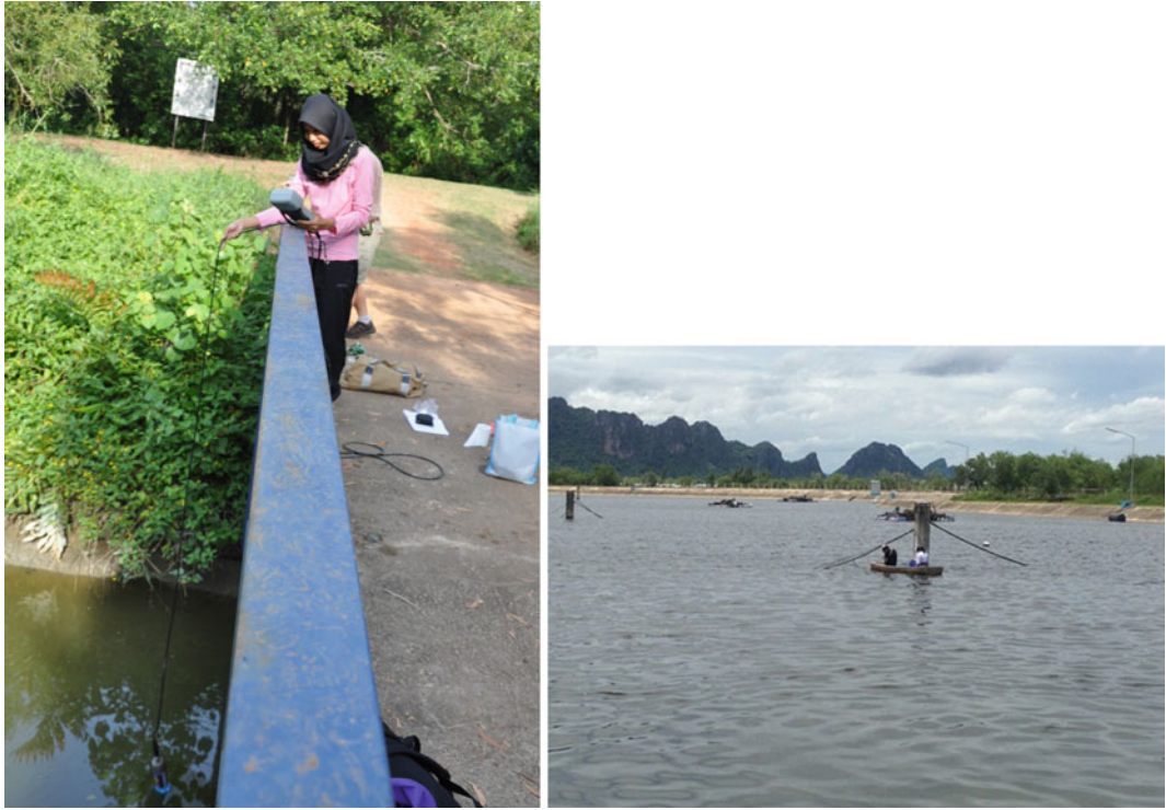
Fig. 6.6 Spot measurements in a canal, Selangor Nature Park, Malaysia (photo courtesy of Firuza Begham Binti Mustafa), and profiling from a boat in an aerated lagoon wastewater treatment facility, Cha am, Thailand (photo courtesy of Shwesin Koko)
