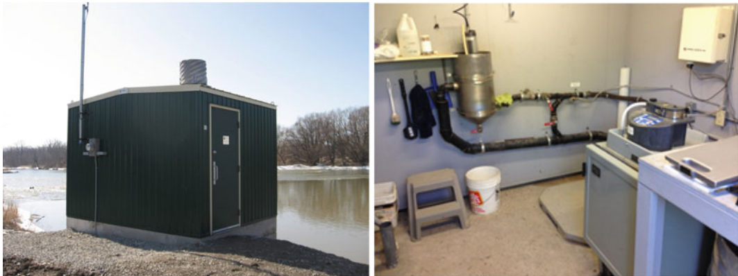
Fig. 6.5 Monitoring station housing the datasonde and automated water sampler at the Grand River in Ontario, Canada (left). Inside the monitoring station, attached to the wall is the stainless-steel tank containing the datasonde and the ISCO automated water sampler in the foreground (right) (photos by the authors)
