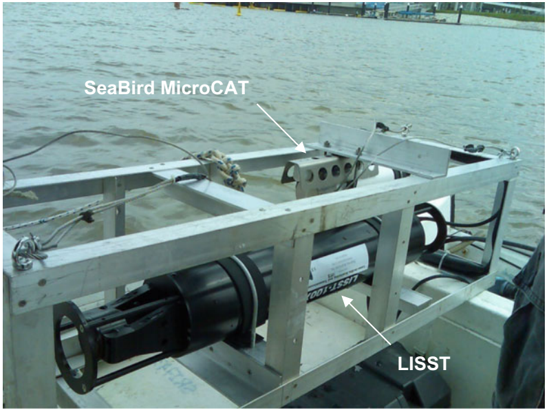
Fig. 6.8 SeaBird MicroCAT profiler and Laser In Situ Scattering Transmissometry (LISST, for particle size and volumetric concentration of particles varying with depth) system being deployed from a boat in a Singapore reservoir (photos by the authors)
