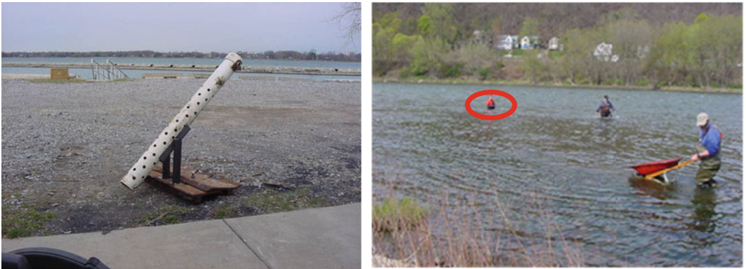
Fig. 6.3 PVC pipe (with holes) fixed to a backhoe tread for weight (left) and installed in the Allegheny River, Pennsylvania (right). Datasonde is circled in red (photos by the authors)
