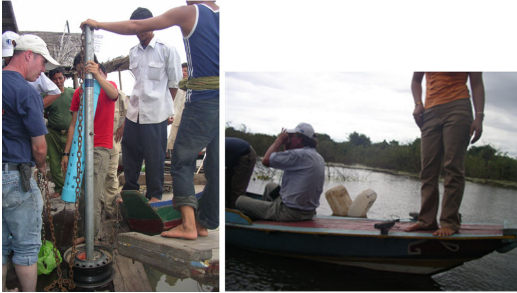
Fig. 6.4 Datasonde deployment in the flooded forest fringe of the Tonle Sap Lake, Cambodia, with the bottom unit (left) and the surface deployment floated with empty water containers (right) (photos by the authors)
