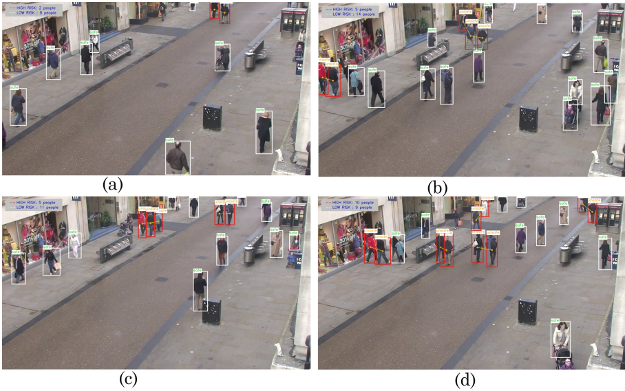
Fig. 4. Output of the proposed physical distancing system. Here, (a), (b), (c), (d) represents the low risk, lower medium risk, medium risk and high risk. (Color figure online)
