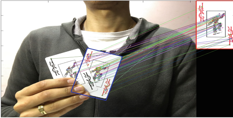
Fig. 13. Object recognition with an occlusion under uncontrolled conditions with two similar objects.
