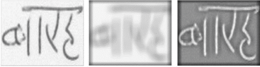
Fig. 3. Illustrates the difference of Gaussian filtering technique, from left-to-right, first image filtered with \sigma = 1 second image filtered with \sigma = 40 . Finally, resulting third image obtained after subtracting second image from first image.
