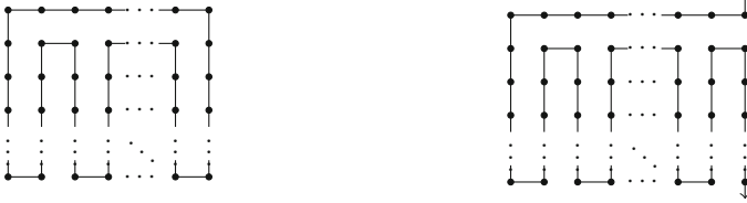
Fig. 2. Feasible Hamiltonian cycles of cost 2(g_1 - 1) when g_1 is even (left) and odd (right).
