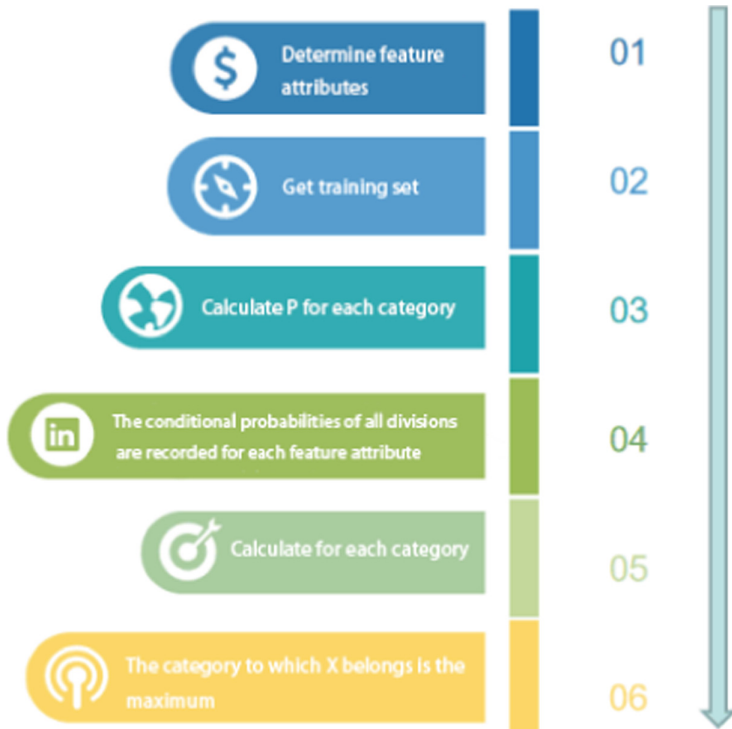
Fig. 3. Flow chart of naive Bayes algorithm.
