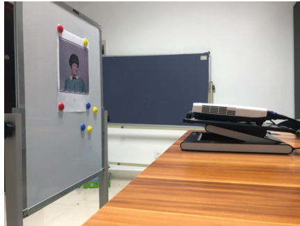
Fig. 6. Experimental system. The left side shows the whiteboard and the test carrier used for the environment, and the projector is placed on the table on the right. The additional magnets (colourful dots for fixing the carrier) are only needed for the sake of the experiment.
