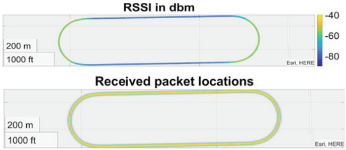
Fig. 33 RSSI and received packets—Baseline (no interference)
