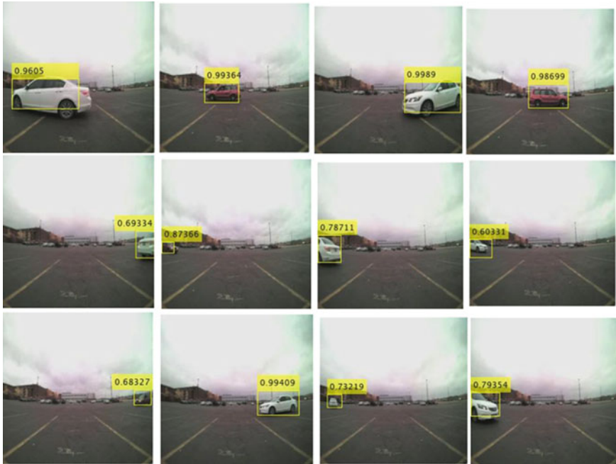
Fig. 12 Vehicle detection results with VGG16-faster R-CNN
