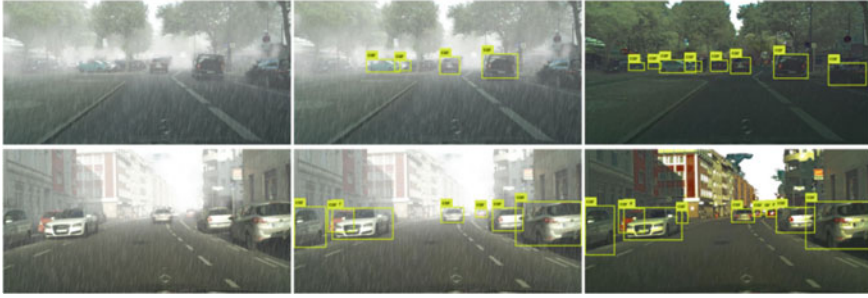
Fig. 15 Object detection results generated by the combination of Yolov3 and JDDNet
