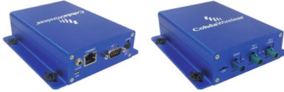
Fig. 4 DSRC Cohda MK5 OBU radios
