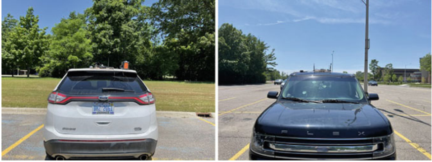
Fig. 4 The pictures of C-V2X transmitter (left) and receiver with beamforming antenna array (right)
