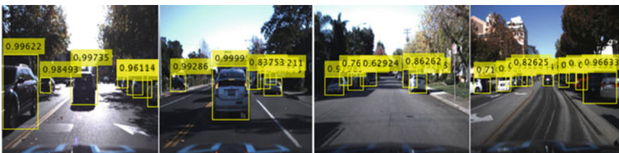
Fig. 11 The validation results of the vehicle detection system on the Udacity vehicle data set
