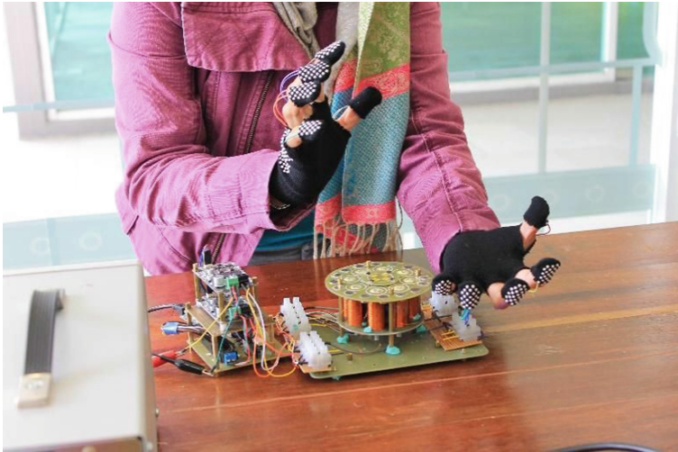
Fig. 7. Haptic gloves in combination with a tower of electromagnets. The electromagnets are arranged throughout the tower to provide dynamic magnetic frictions. (© Predrag K. Nikolic. Photo: Predrag K. Nikolic)
