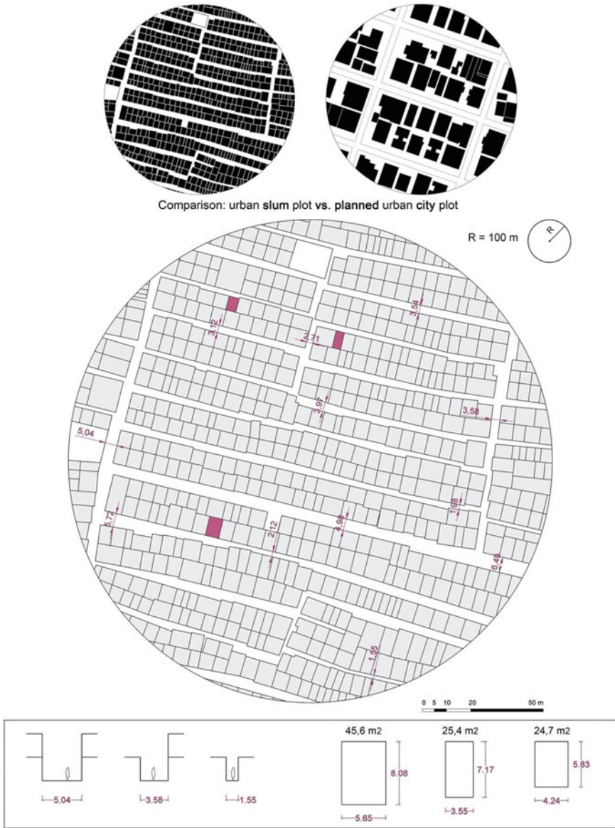
Fig. 27.7 Density comparison. A detailed plan of the slum: the dimension of the houses and streets. [Author's graphic]
