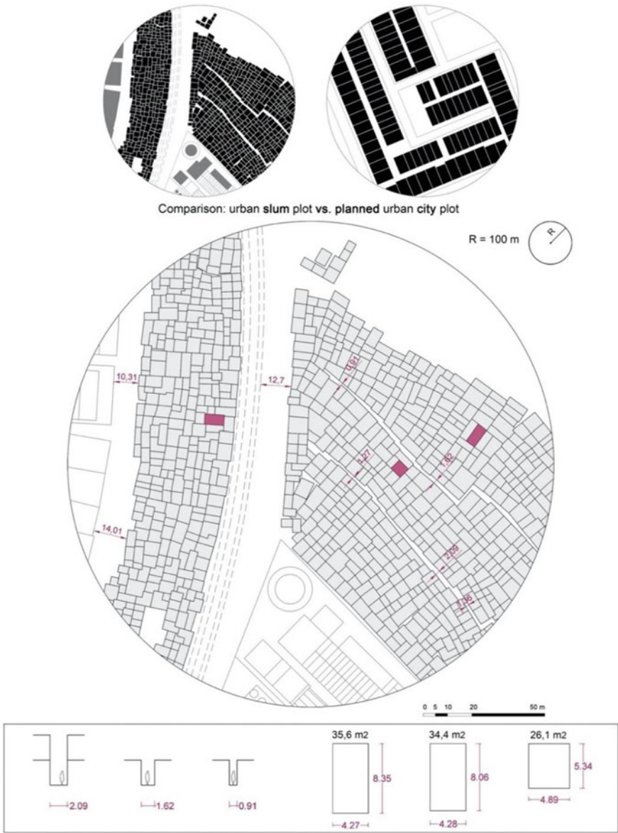
Fig. 27.13 Density comparison. A detailed plan of the slum, dimensions of the houses and streets. [Author's graphic]
