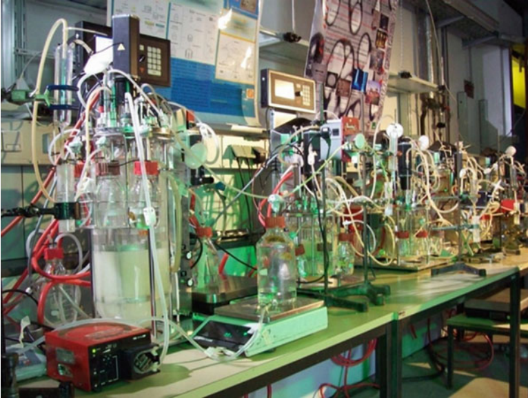
Fig. 3 Multistage bioreactor cascade for high-throughput PHA biosynthesis, financed by BASF SE, in operation at Graz University of Technology, Austria. (Own picture M. Koller)
