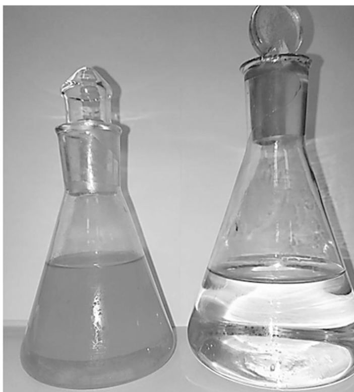
Fig. 11.6 FAME with the addition of biocidal additive (right) and without it (left)
