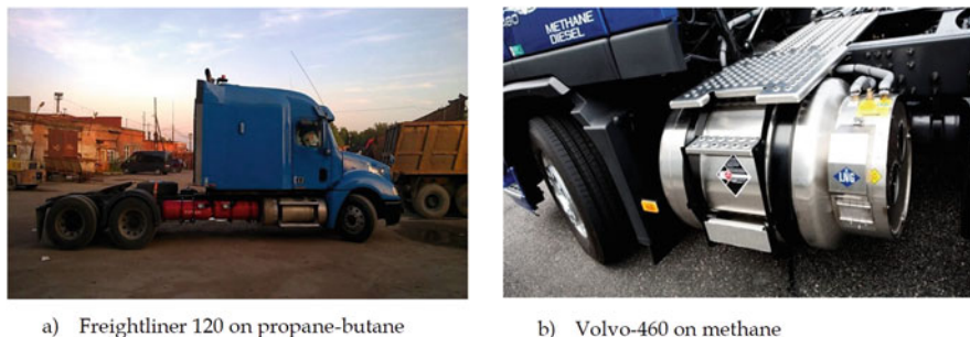
Fig. 10.1 Transport vehicles powered with gas fuels. (a) Freightliner 120 on propane-butane. (b) Volvo-460 on methane
