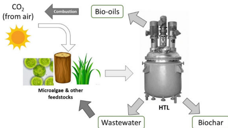
Fig. 28.2 Circular aspects of bio-oil production from microalgae
