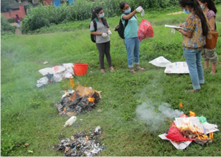
Fig. 25.5 Measurement of sample mass of trash and burning
