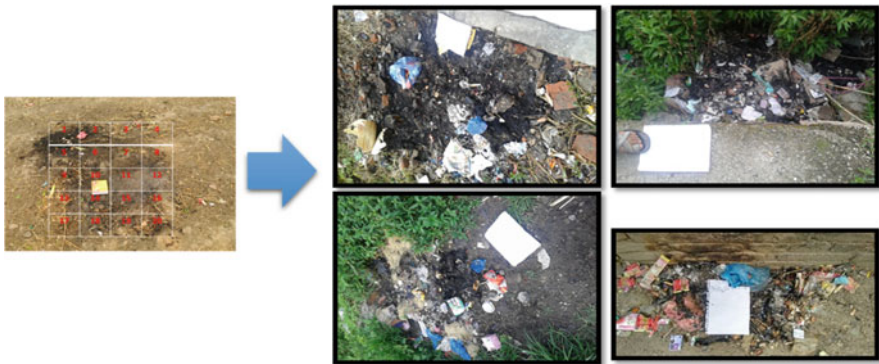
Fig. 25.7 Quadrature method to estimate fraction of MSW burning at disposal sites
