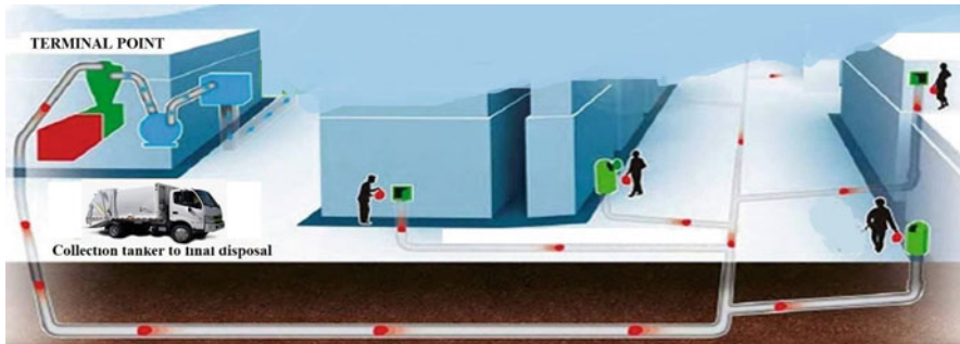
Fig. 7.15 Basic layout of a waste pneumatic collection system (Waste Collection Report 2007)
