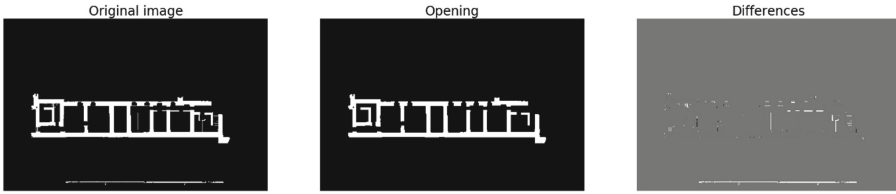
Fig. 3. Discarding thin structures: original wall image (left), after processing (center), difference image (right).
