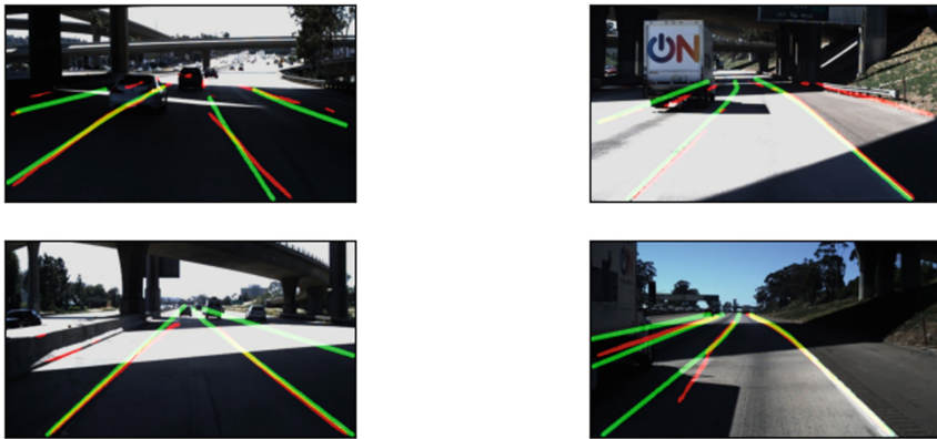
Fig. 1. Lane detection using LaneNet [6] under driving scenarios with shadows, light reflections and lane occlusions from the TuSimple dataset. Green lanes represent the ground truth and red, the ones inferred by the network.
