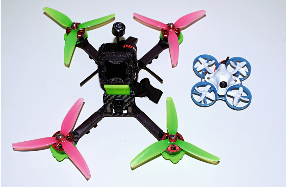
Fig. 2. Two types of FPV drones: 5-in. outdoors drone (left), and 65 mm designed for indoor use (right).
