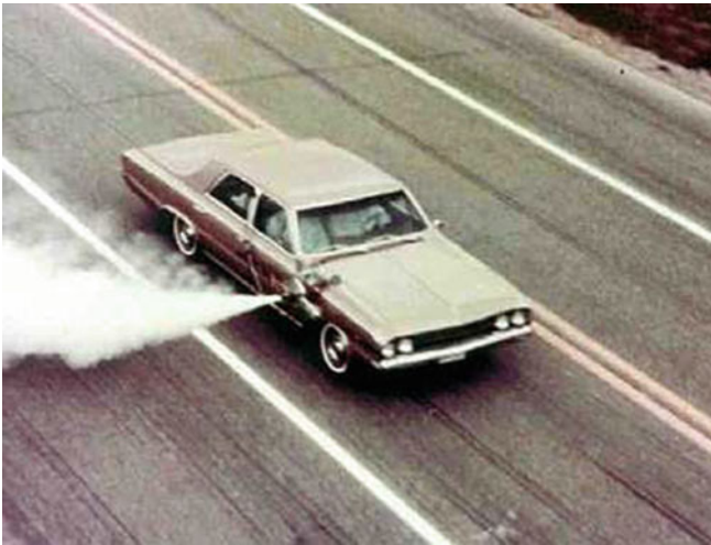
Fig. 7.68 Lateral force applied by means of a rocket (General Motors Corporation, circa 1960)
