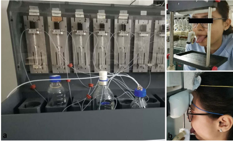
Fig. 3 Stimulation for the recording of gustatory event-related potentials. (a) Stimulating device to obtain gustatory event-related potentials (GERP) (Gustometer GU001; Burghart instruments, Wedel, Germany). The fast syringes (top) are operated to produce precisely defined amounts of liquid which is drawn from the bottles. (b) Subject with extended tongue at gustometer outlet during GERP recording. The tastants are sprayed onto the tongue embedded in a constant sprays of tasteless liquid (artificial saliva)
