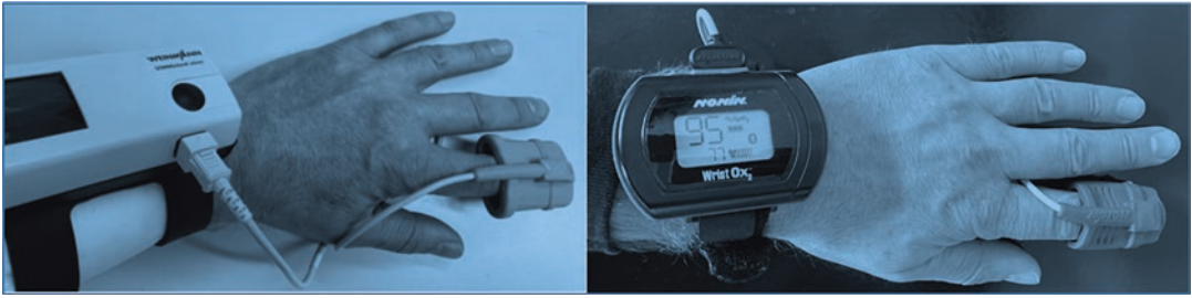
Fig. 9.2 Example of simplified HSAT devices (left panel, SOMNOcheck micro CARDIO , Weinmann/Löwenstein Medical SE & Co. KG; right panel, WristOx 2 Model 3150 , Nonin Medical, Inc.) using photoplethysmographic sig-
